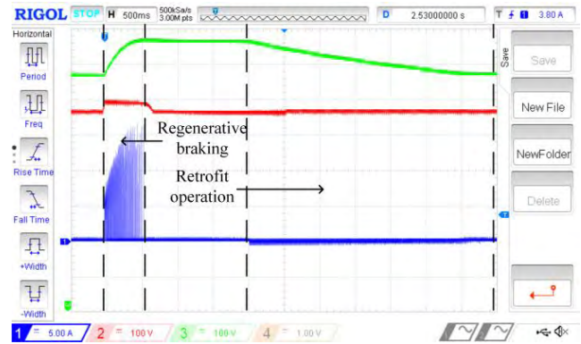
FIGURE 14. Operation of the bidirectional DC-DC converter during a motor stop and operation for energy recuperation: capacitor bank voltage (upper waveform, 100V/div), DC-bus voltage (middle waveform, 100V/div) and inductor current (lower waveform, 5A/div).
