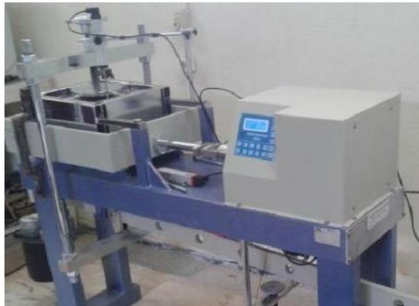
**Figure 2. Large direct shear test apparatus**
