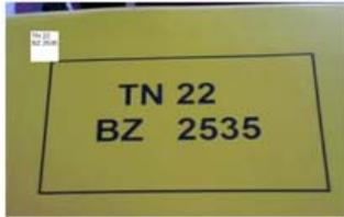
**Fig. 10. The output of the DNN printing the alpha numeric characters**
