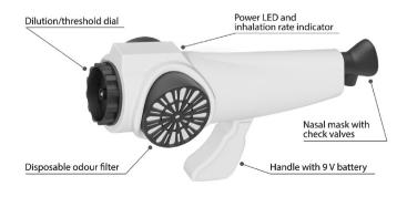
Fig. 1. Basic elements of field olfactometer.
