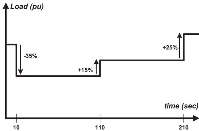
Fig. 12. Load curve used for all loads in the test system.
