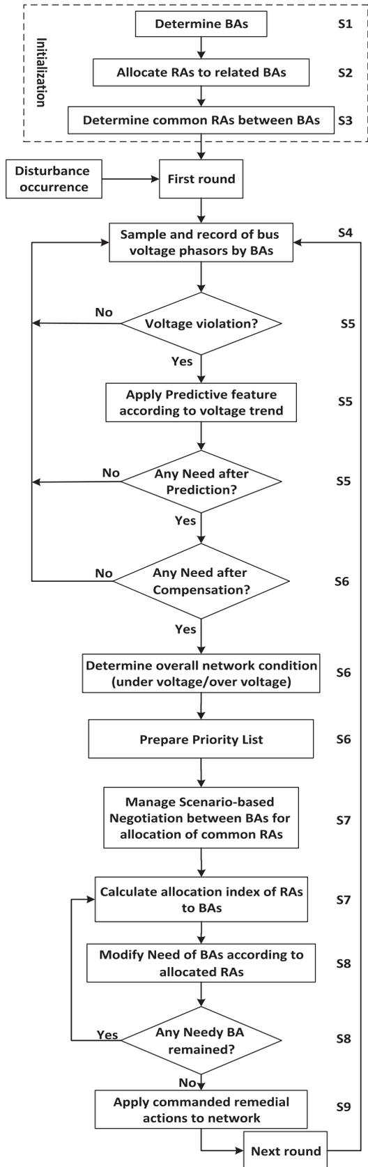
Fig. 3. The flowchart of the proposed voltage control scheme.
