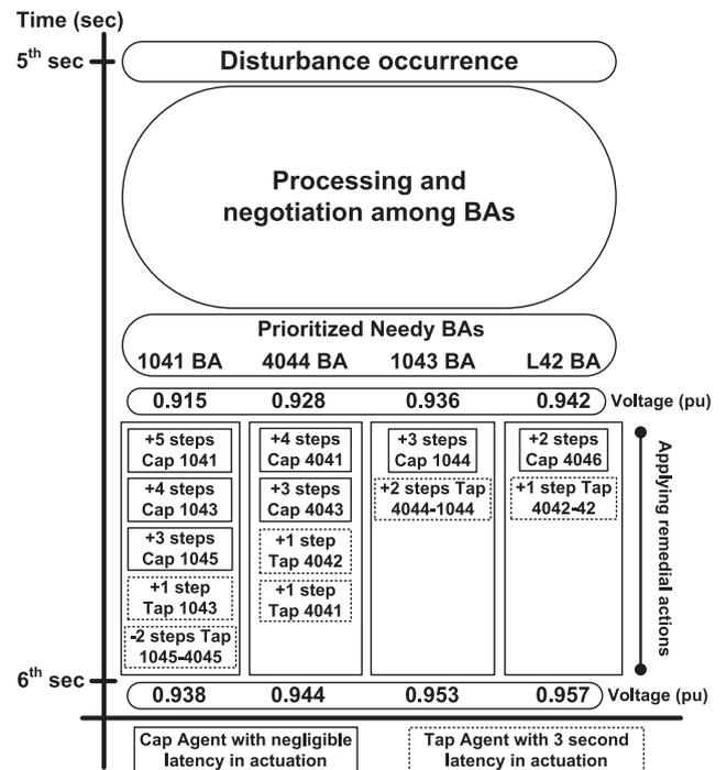
Fig. 10. The time line of applying the first round of the proposed scheme.
