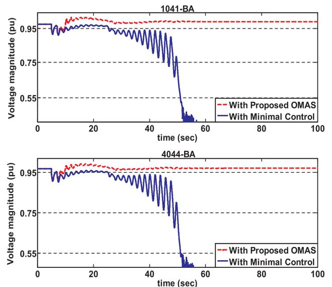
Fig. 15. The performance of OMAS against voltage collapse.
