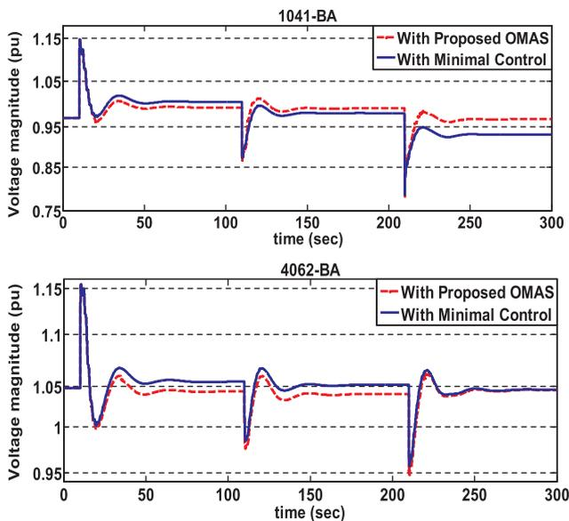
Fig. 13. Voltage phasors of two BAs in confronting with load variations according to the load curve of Fig. 12.
