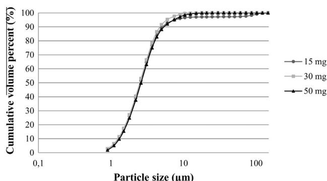
Fig. 4. Effect of the tobramycin dose on the dispersion efficiency of the Cyclops. PSDs in the delivered aerosols from the Cyclops operated at 4 kPa for doses of 15, 30 and 50 mg pure spray dried tobramycin (TOB) measured by laser diffraction analysis using an INHALER 2000 adapter and a HELOS BF laser diffractometer.
