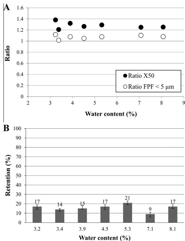
**Fig. 6.** Effect of the water content on the dispersion efficiency (A) and retention (B) for 30 mg pure spray dried doses dispersed with the Cyclops at 4 kPa. The closed circles in figure A show the ratio of  $X_{50}$  for the primary PSD to the  $X_{50}$  for the aerosol from the Cyclops and the open circles show this ratio for the FPF < 5 μm as function of the water content in the samples. In figure B for the inhaler retention, the error bars indicate the minimum and maximum values measured.
