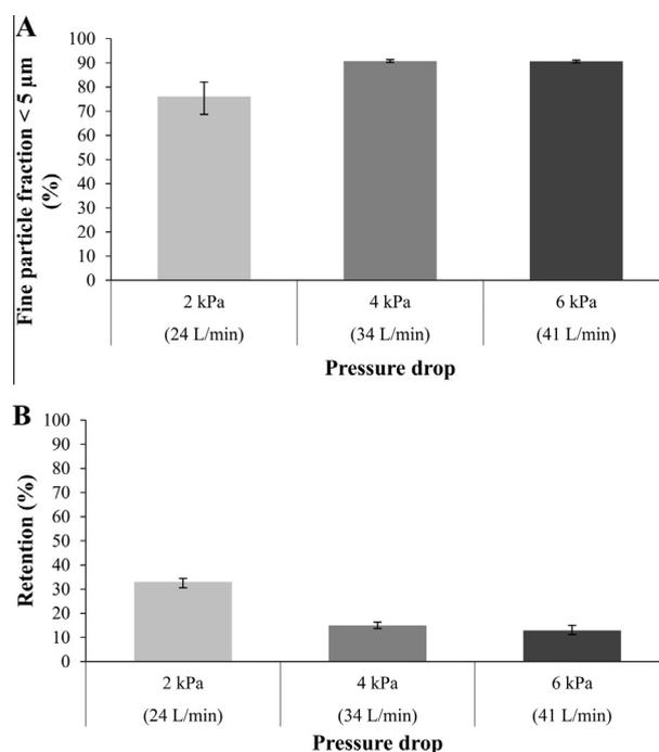
Fig. 5. Effect of the pressure drop on the dispersion (A) and retention (B) of a 30 mg tobramycin dose in the Cyclops. Comparison of the FPF < 5  $\mu\text{m}$  (A) and the retention values (B) for doses of 30 mg pure spray dried tobramycin (TOB) at 2, 4 and 6 kPa in the Cyclops. The error bars indicate the minimum and maximum values found.
