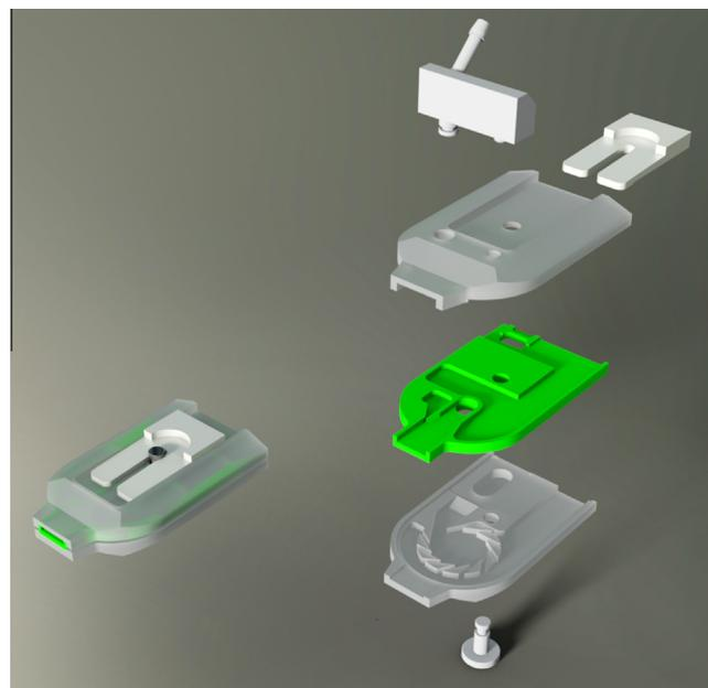
**Fig. 1.** Presentation of the Cyclops disposable DPI for spray dried aminoglycosides. On the left side the assembled Cyclops that was used for the *in vitro* evaluation programme and on the right side an exploded view of the Cyclops that was used in a pilot study and was modified to be able to measure the pressure drop across the Cyclops.
