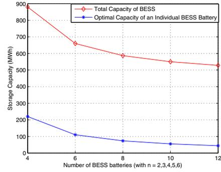
Fig. 5. The optimal BESS capacity trend vs number of batteries in a BESS.
