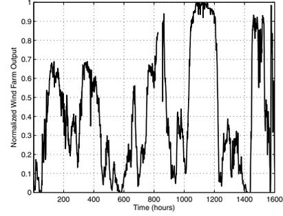
Fig. 2. Typical wind farm's power profile.
