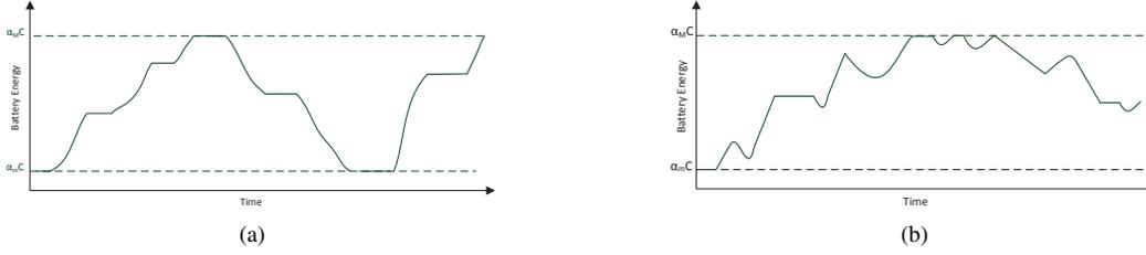
Fig. 3. Charging/discharging characteristics of a BESS (a) A monotonic charge/discharge. (b) A charge/discharge without the monotonicity requirement.
