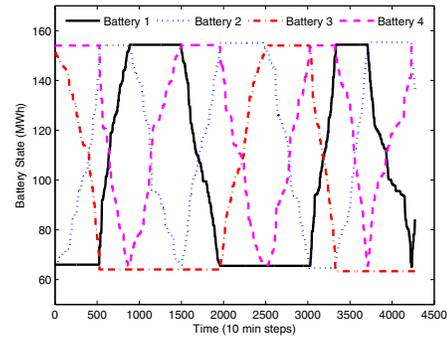
Fig. 6. Monotonic charging/discharging of BESS batteries within 30% - 70% operation band of optimal capacity each with fast rates.
