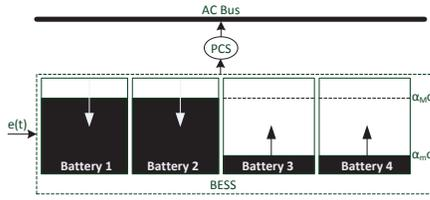
Fig. 4. The charging/discharging structure of the BESS.
