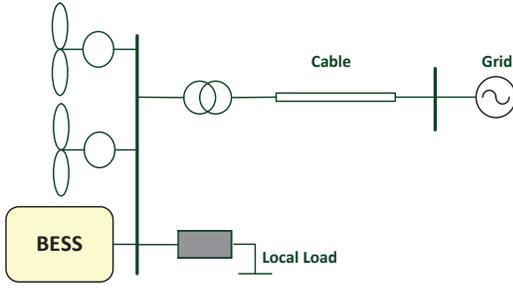
Fig. 1. A grid-connected wind farm with a BESS.
