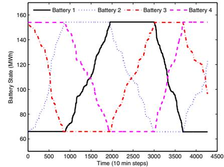
Fig. 7. Monotonic charging/discharging of BESS batteries within 30% - 70% operation band of optimal capacity each with slow rates.
