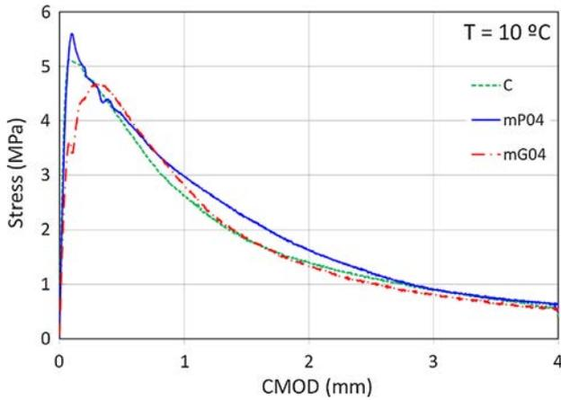
Fig. 7. Stress – CMOD curves of FRAC incorporating microfibers.
