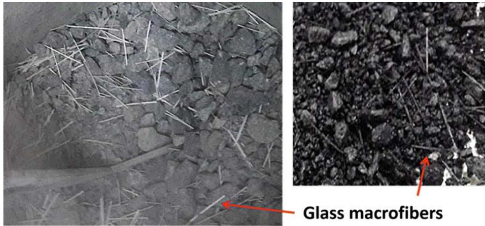
Fig. 2. FRAC mixing. Fiber incorporation and mixture aspect.
