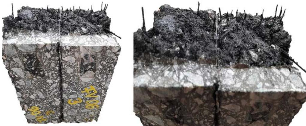
Fig. 12. View of fracture surface after bending tests.
