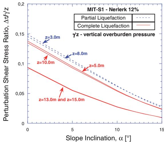
Figure 9. Stability charts for the Nerlerk berm.
