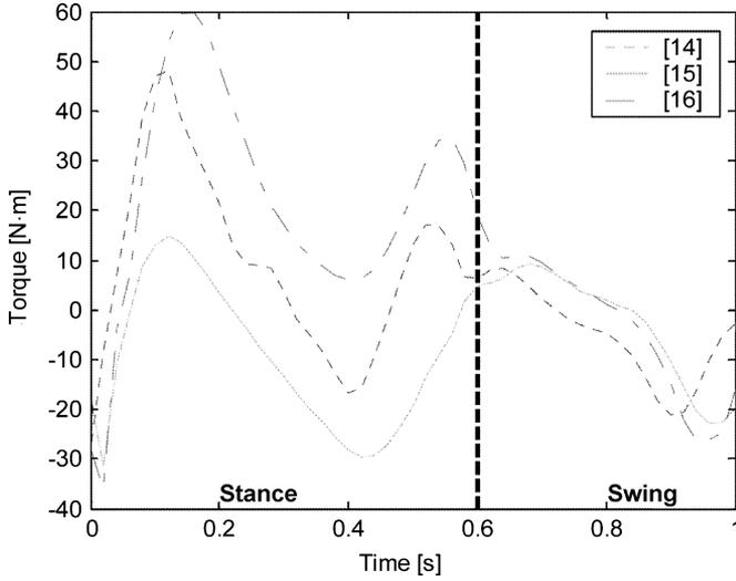
Fig. 10. Adjusted CGA data of the knee flexion/extension torque. An initial  $-35$  N·m flexion torque is required at heel strike, followed by large extension torques ( $\sim 60$  N·m) to keep knee from buckling in stance phase.
