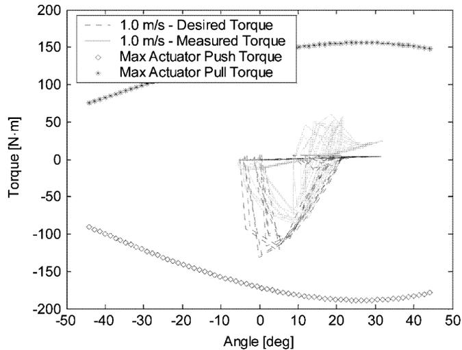
Fig. 27. Ankle torque versus angle data measured from BLEEX walking.
