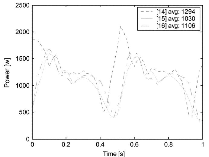
Fig. 20. Hydraulic power requirement for BLEEX walking.
