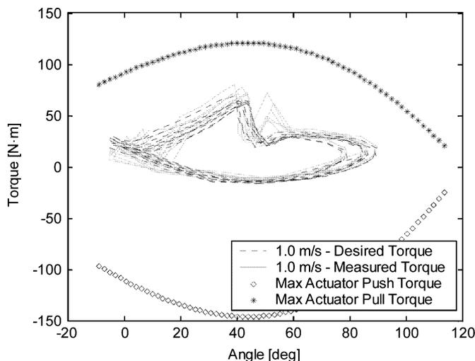
Fig. 29. Hip torque versus angle data measured from BLEEX walking.
