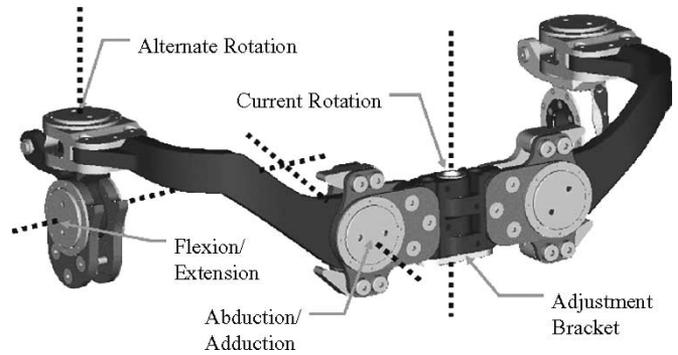
Fig. 2. BLEEX hip DOF (back view). Only the rotation axis does not pass through the human hip ball and socket joint. The adjustment bracket is replaceable to accommodate various sized operators.
