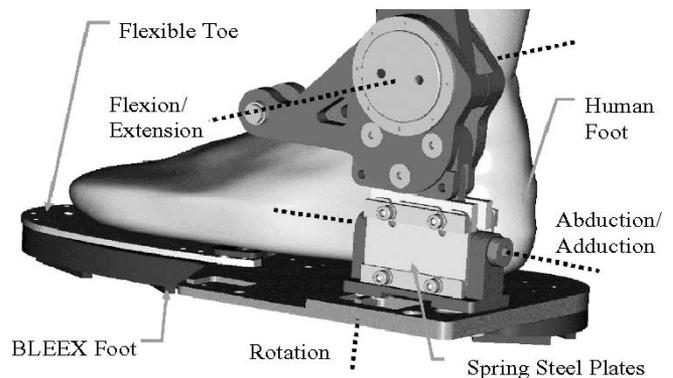
Fig. 3. BLEEX ankle DOF. Only the flexion/extension axis passes through the human's ankle joint. Abduction/adduction and rotation axes are not powered, but are equipped with appropriate impedances.
