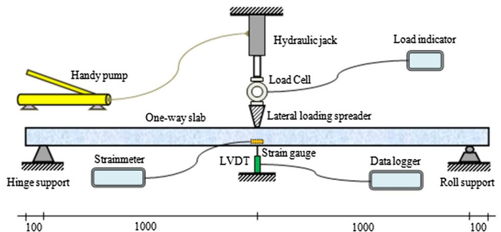
**Fig. 4** Testing setup of instrumentations
