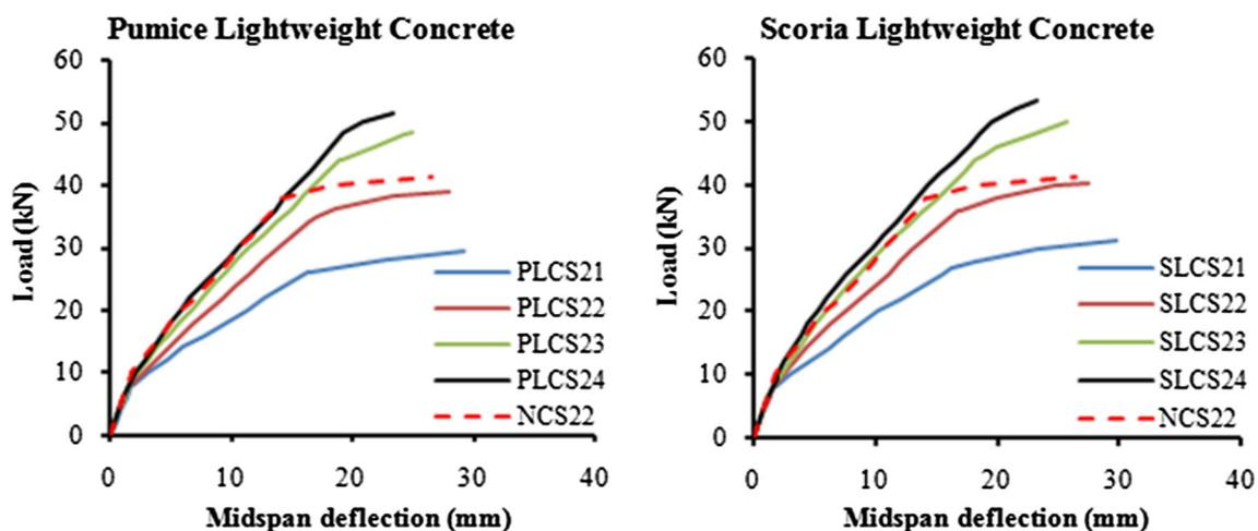
**Fig. 5** Load-midspan deflection diagrams
