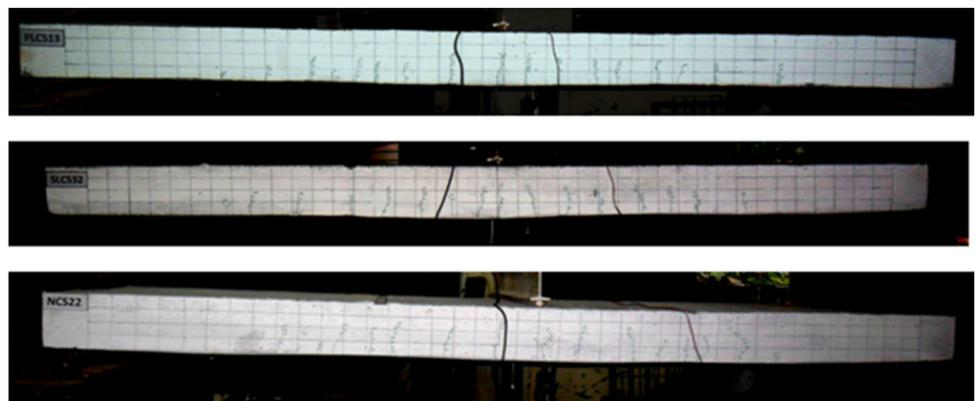
cracks on the sides of pumice lightweight concrete one-way slabs ranged (13–21), while for scoria lightweight concrete one-way slabs ranged (12–20). For the second compressive strength and reinforcement ratio, the number of cracks of the pumice lightweight concrete one-way slab is greater than the control, while the scoria lightweight concrete one-way slab is the same number as the control.
