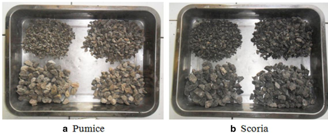
Fig. 1 Grading of pumice and scoria coarse aggregates
