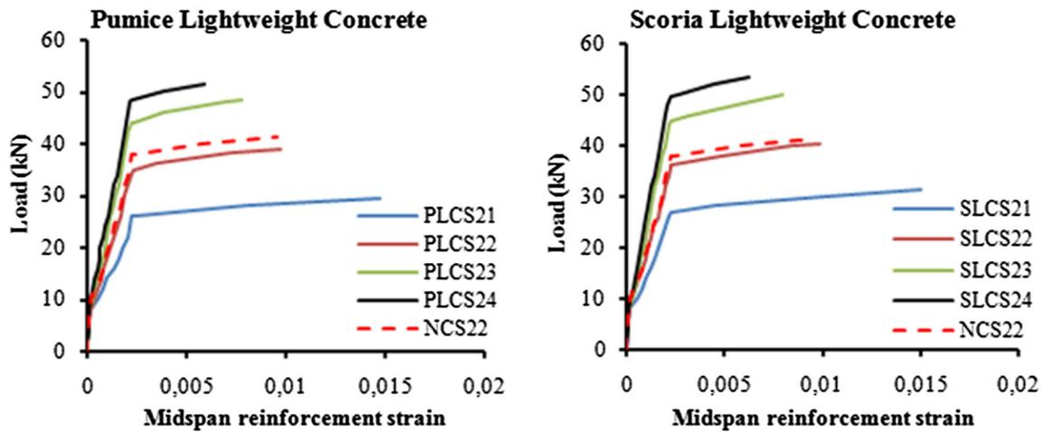
Fig. 7 Load-midspan reinforcement strain diagrams
