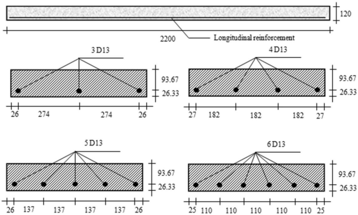
Fig. 2 Detail of reinforced concrete one-way slabs
