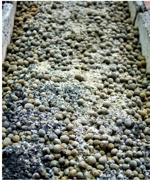
Fig. 2. Burned aggregate with rest of the ignition layer.
