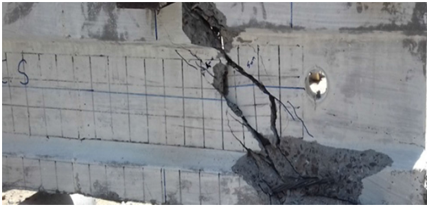
Fig. 14 Crack patterns of P1 beam
