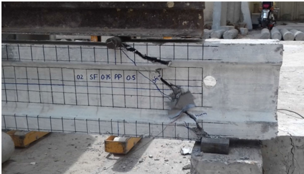
Fig. 15 Crack patterns of P2 beam
