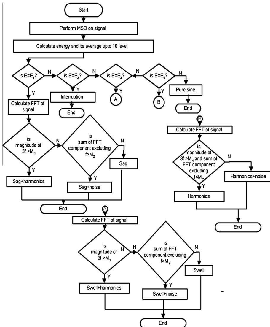
**Fig. 12.** Integrated DWT–FFT rule based system flow chart.
