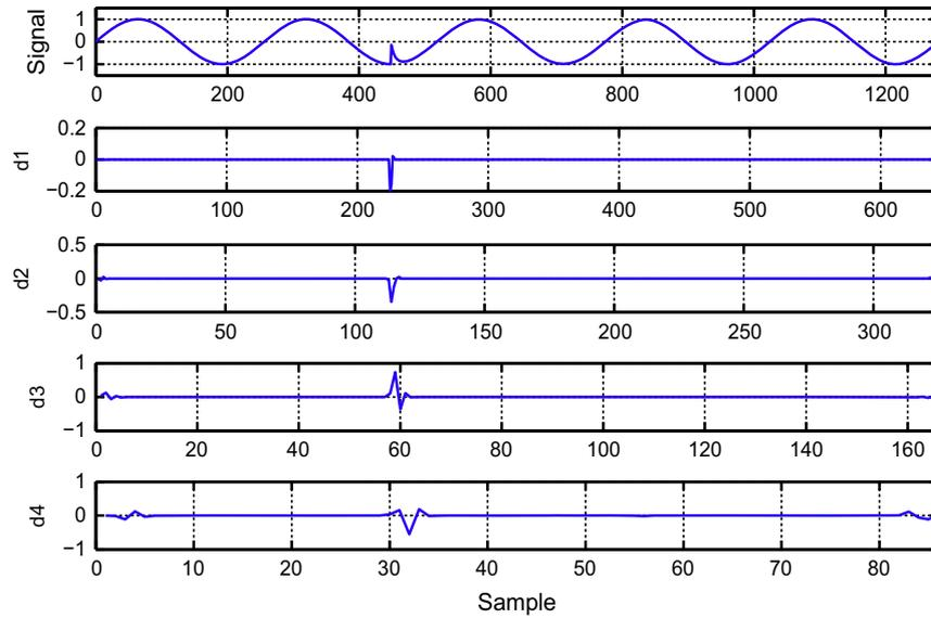
Fig. 7. Four level squared DWTC decomposition for detection of capacitor switching.
