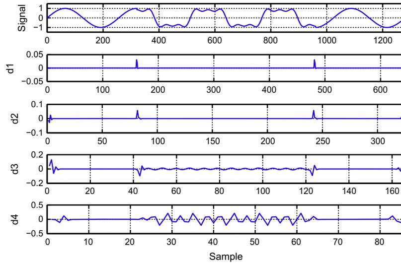
Fig. 4. Four level squared DWTC decomposition for detection of harmonics.
