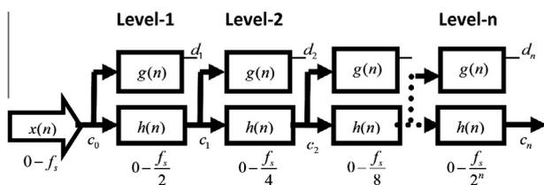
Fig. 1. Typical three level MSD based on DWT.
