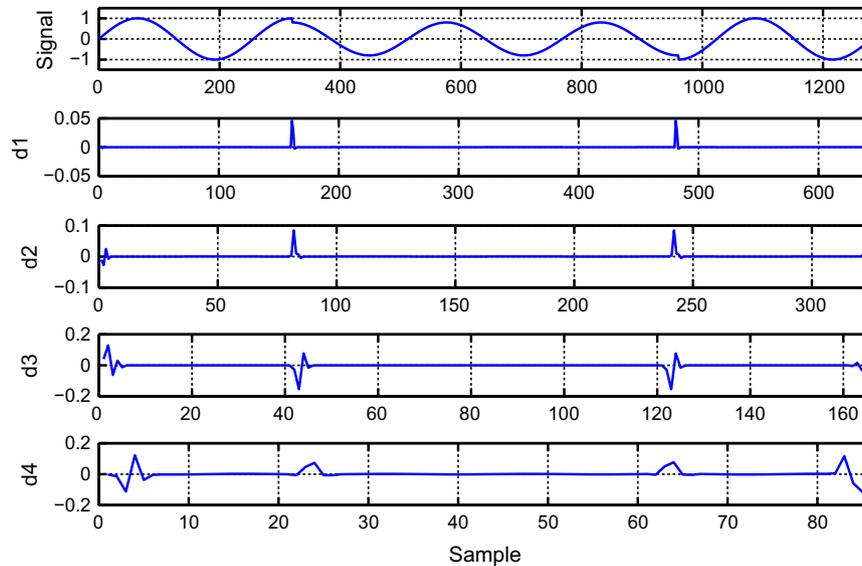
Fig. 2. Four level squared DWTC decomposition for detection of voltage sag.
