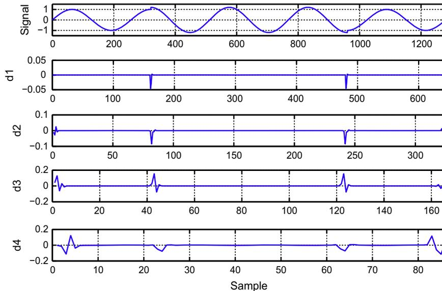
Fig. 3. Four level squared DWTC decomposition for detection of voltage swell.
