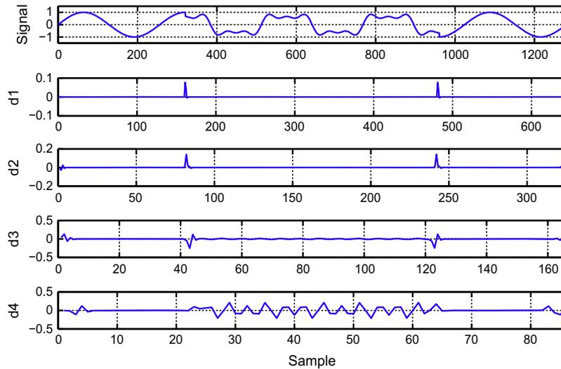
Fig. 6. Four level squared DWTC decomposition for detection of sag + harmonics.
