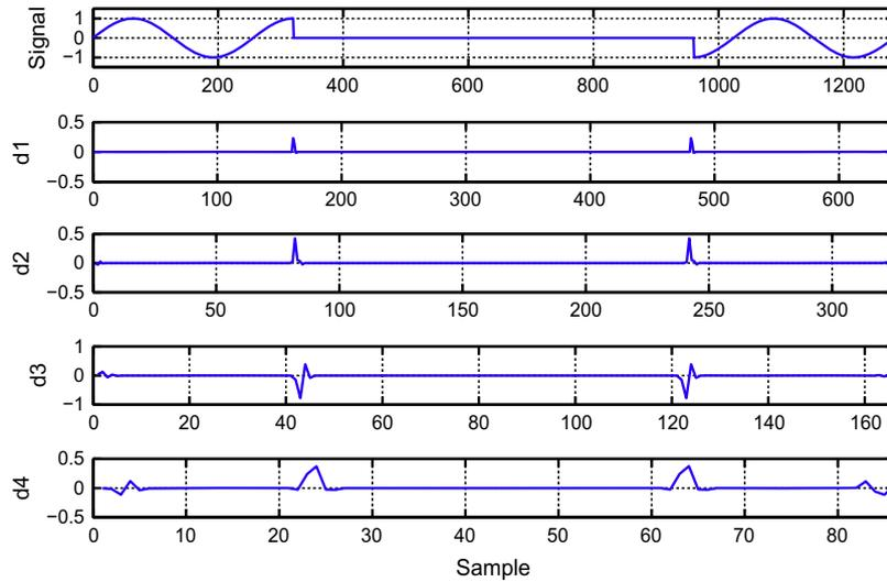
Fig. 5. Four level squared DWTC decomposition for detection of interruption.
