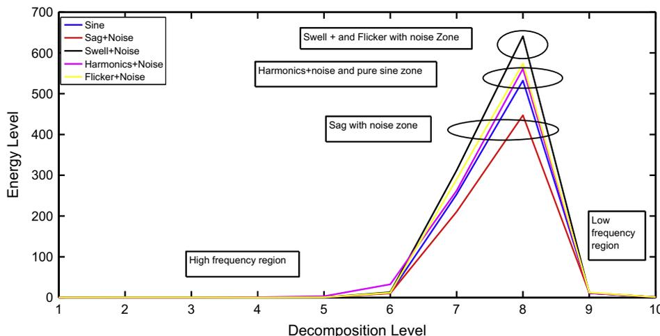
Fig. 10. MRA curve for the comparison of energy levels in sine wave and other power quality disturbances during MSD under noisy environment.
