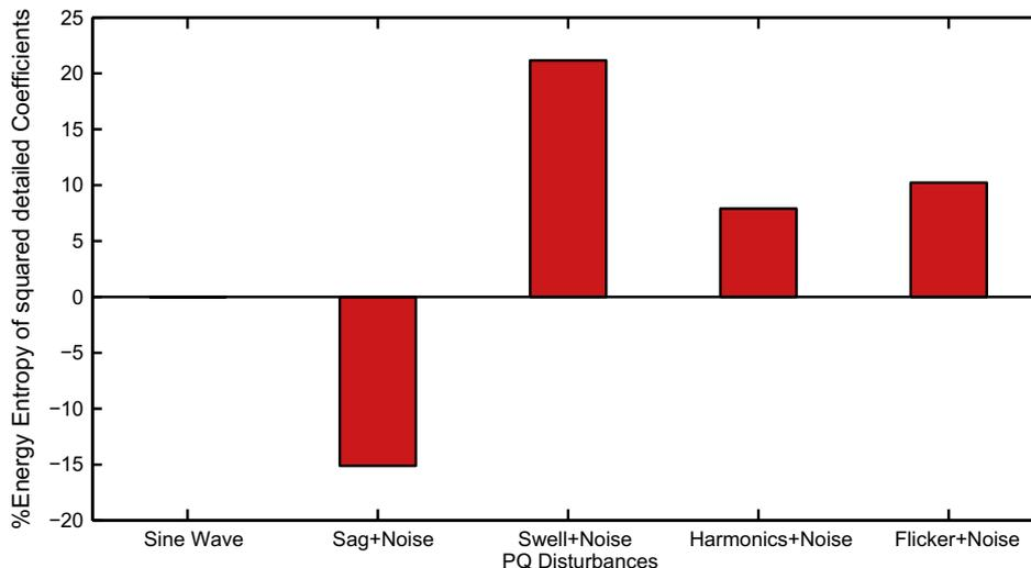
**Fig. 11.** Bar chart for percentage energy entropy of squared DC with noise.
