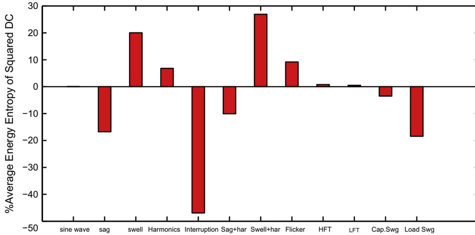
Fig. 9. Bar chart for percentage energy entropy of squared detailed coefficients.
