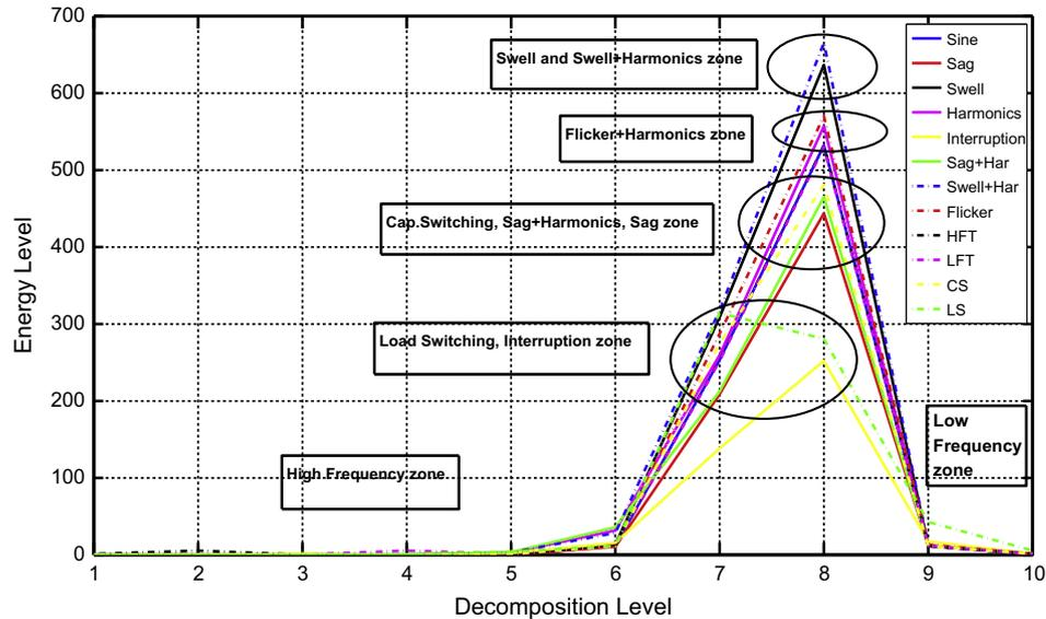
Fig. 8. MRA curve for the comparison of energy levels in sine wave and other power quality disturbances during MSD.
