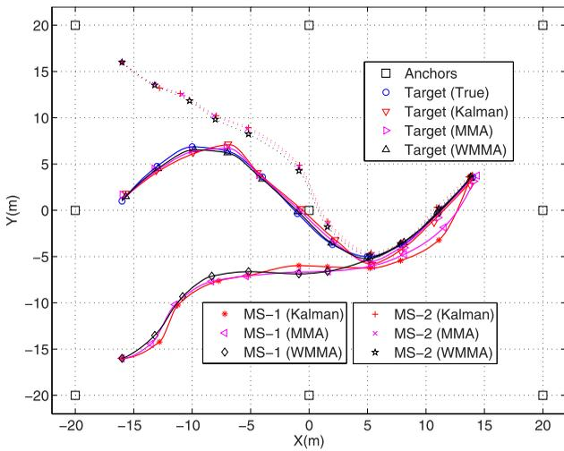
Fig. 7. Comparison of the tracking under different trajectory estimation algorithms.
