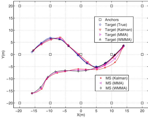
Fig. 3. Comparison of the tracking under different trajectory estimation algorithms.
