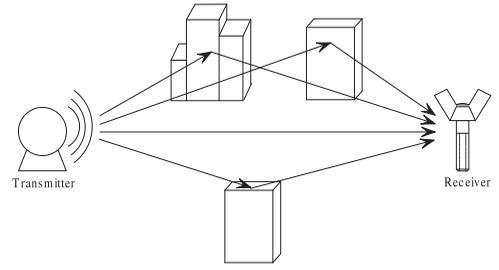
Fig. 1. Illustration of the signal transmission path from the transmitter to the receiver.
