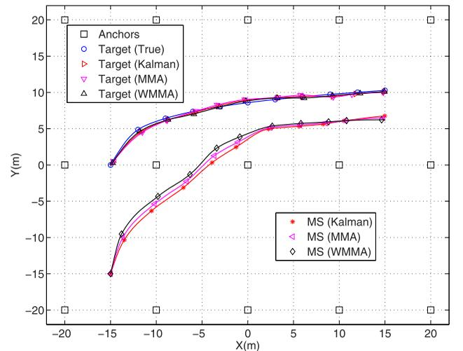
Fig. 6. Navigation to keep a constant distance under different trajectory estimation algorithms.
