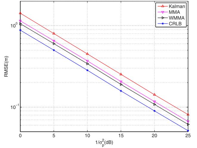
Fig. 5. The average RMSE of the target trajectory estimation under Kalman, MMA, and WMMA algorithm.
