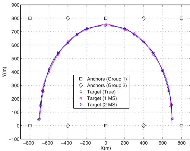
Fig. 10. Comparison of the tracking under different number of mobile sensors under circular trajectory.
