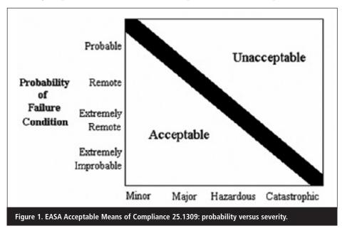
fort for the pilots and physical distress to others, as shown in **Figure 1**. Such failures are not expected to occur in each aeroplane, but may occur several times during the total life of a number of aircraft of type.
