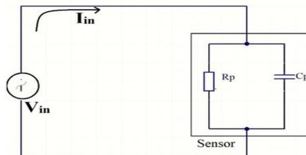
Figure 3: Equivalent circuit of Interdigital sensor
