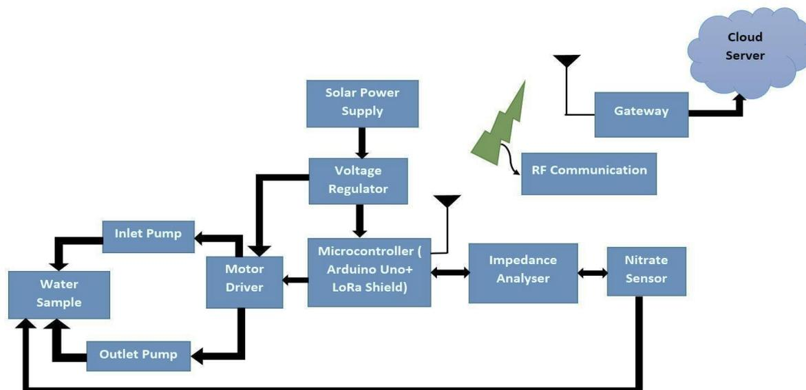
Figure 5: Block diagram of the data transmission
