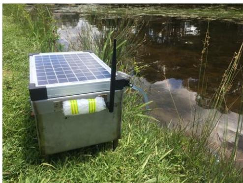
Figure 9: Field installation of the smart sensor node
