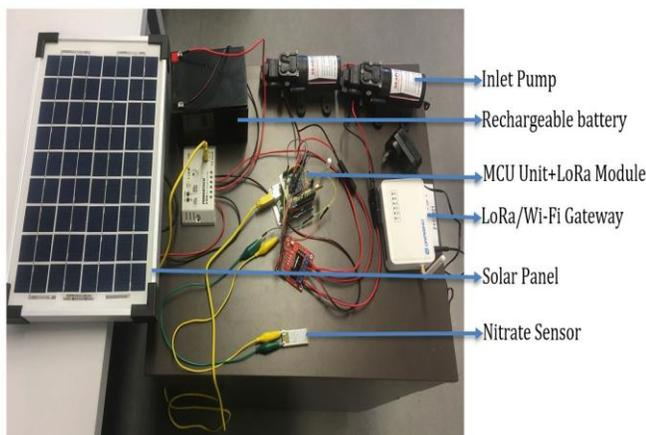
Figure 7: Different parts of the proposed system
