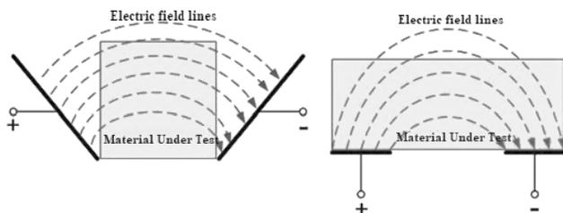
Figure 1: Electric field lines of parallel-plate capacitor and planar interdigital sensor
