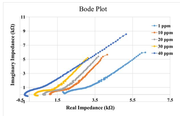
Figure 11: Bode plots for different nitrate concentrations
