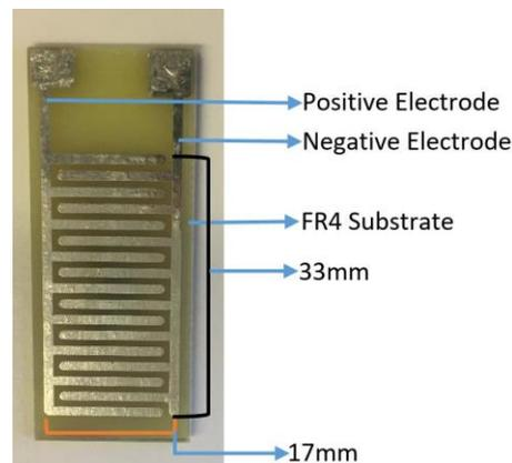
Figure 2: FR4 interdigital sensor and dimensions
