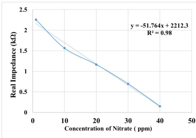
Figure 13: Calibration standard to measure any unknown nitrate concentration
