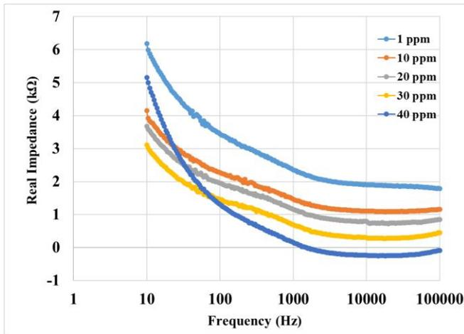
Figure 12: Frequency vs real impedance for different nitrate concentrations
