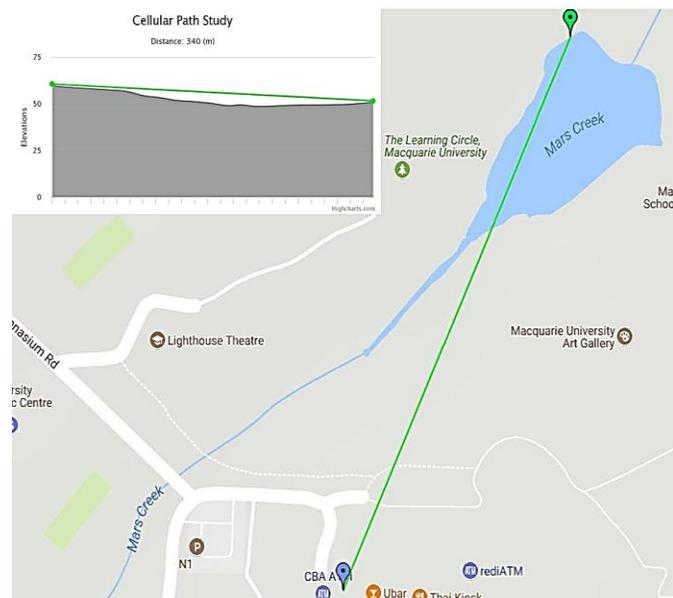
Figure 10: Study location and distance between gateway and the sensor node
