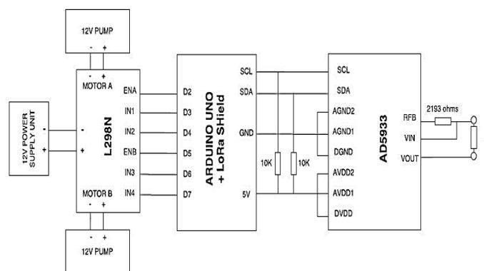
Figure 6: Circuit diagram of the sensing system
