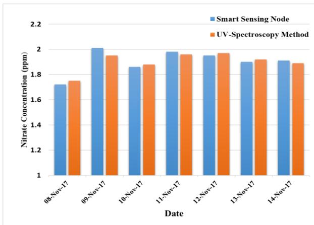
Figure 15: Comparison of daily evolution of nitrate concentration with standard method
