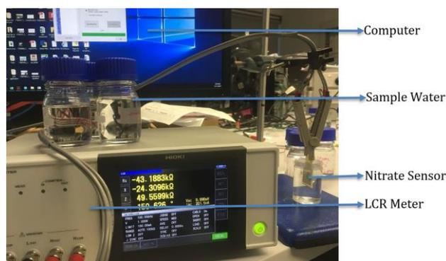
Figure 4 : EIS measurement in laboratory conditions
