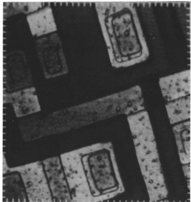
Figure 4. Confocal image of an integrated circuit
