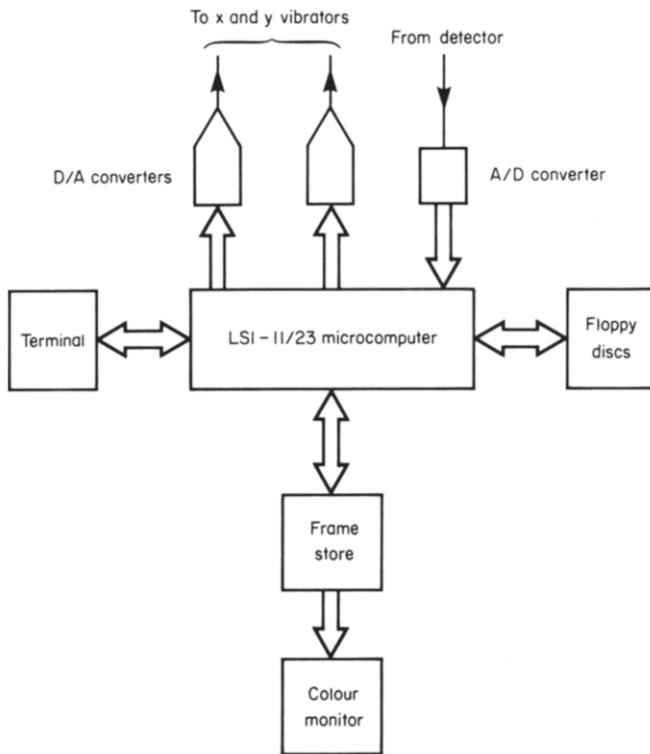
Figure 2. Block diagram of the digital image processing hardware
