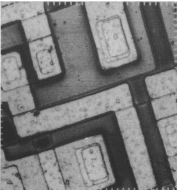
Figure 7. Contrast enhanced autofocus image of an integrated circuit
