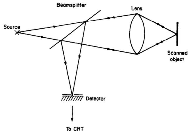
Figure 1. Diagram of a confocal scanning optical microscope
