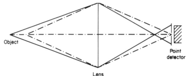
Figure 5. Diagram illustrating the principle of depth discrimination in a confocal microscope
