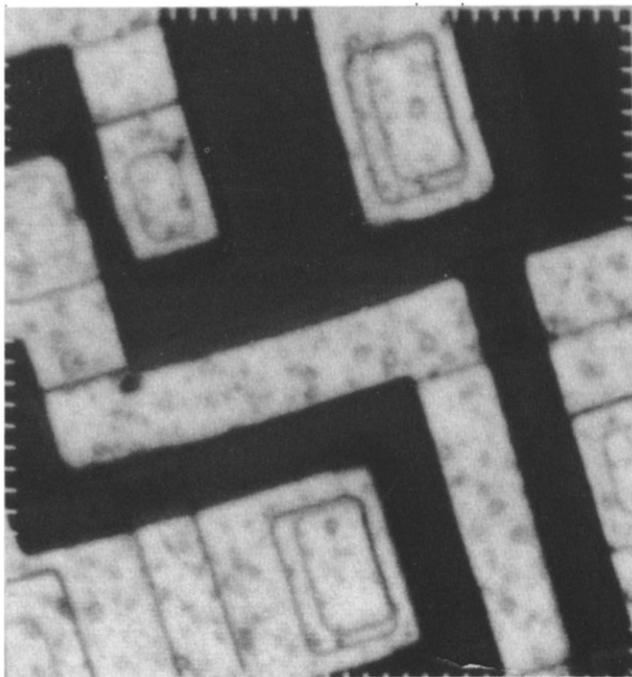
Figure 3. Conventional micrograph of an integrated circuit. Each division represents 4  $\mu\text{m}$
