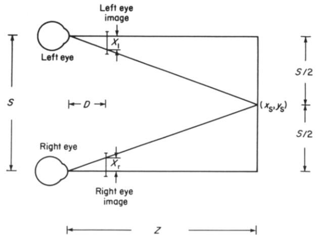
Figure 10. Stereo image forming process
