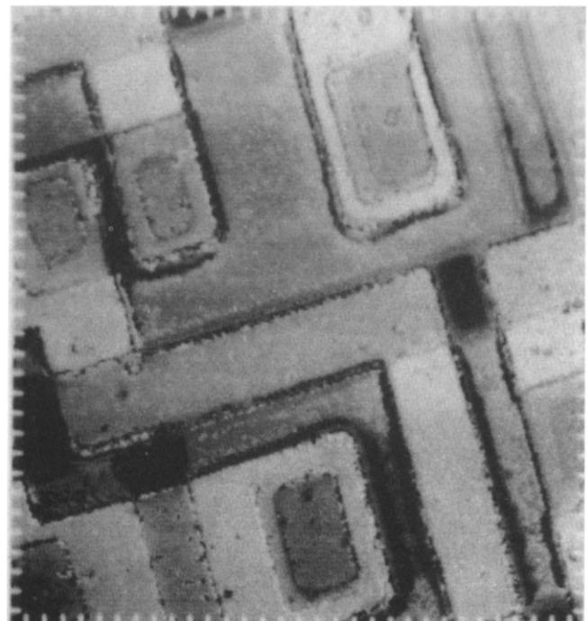
Figure 9. A range image of the integrated circuit. Lighter areas correspond to points closer to the observer
