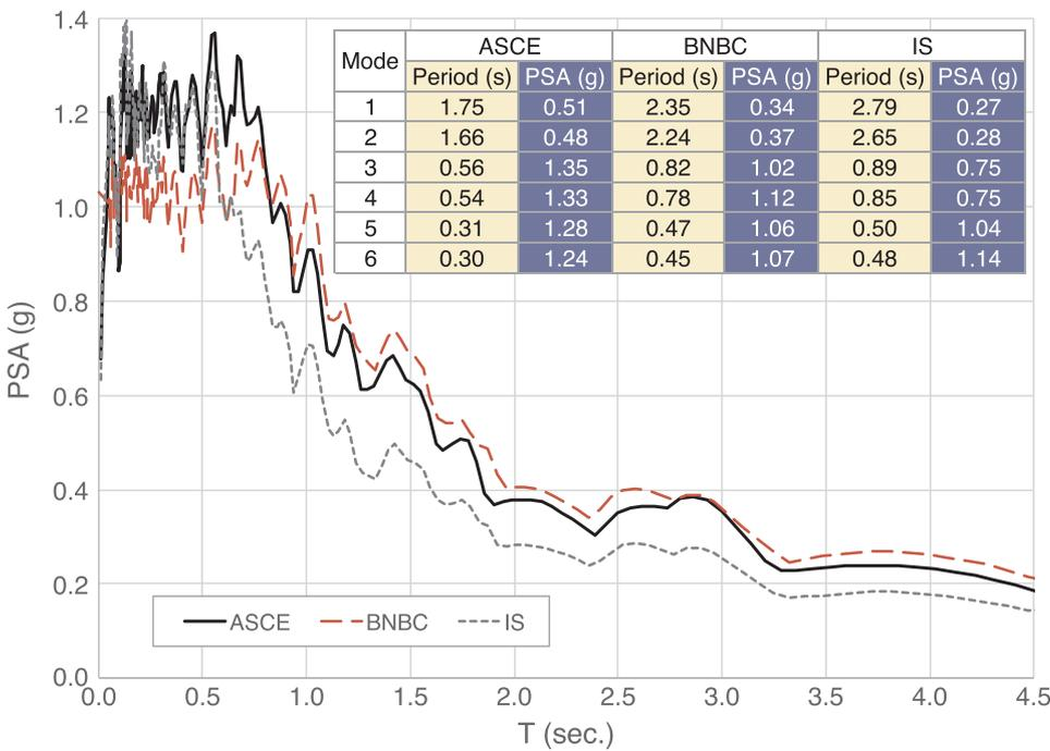
Fig. 11. Comparison of pseudo acceleration response spectra.
