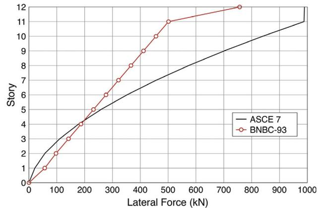
Fig. 2. Comparison of equivalent lateral forces from ASCE 7-10 and BNBC-93.
