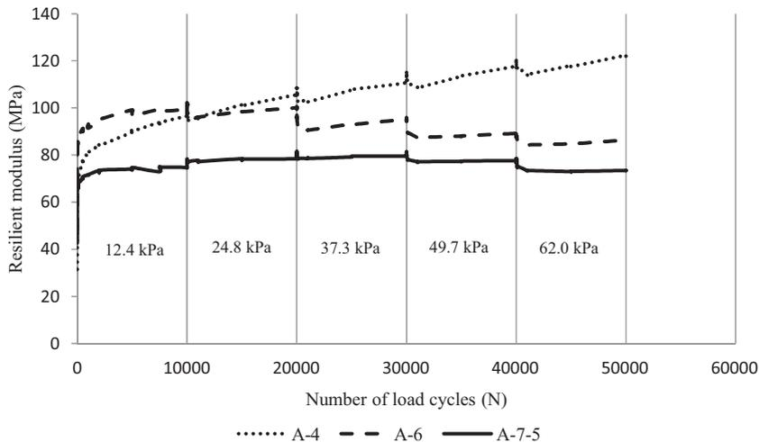
Fig. 2. Resilient modulus values vs. number of load repetitions for different deviatoric stress levels for unstabilised soils.
