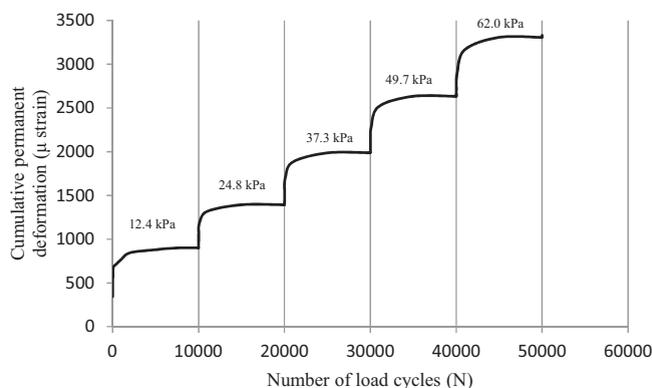
Fig. 4. Relation between accumulative permanent deformation and number of load repetitions in a multi-stage test for unstabilised soil A-4.
