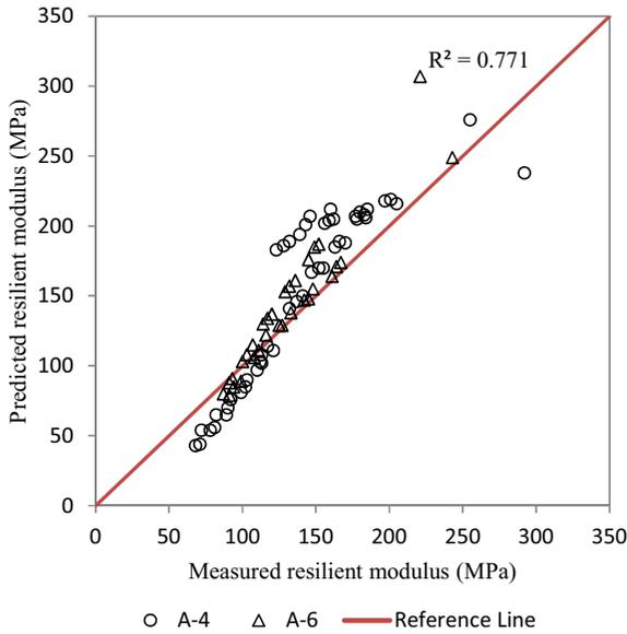
Fig. 1. Relationship between resilient modulus measured from tests and predicted from Eq. (4).
