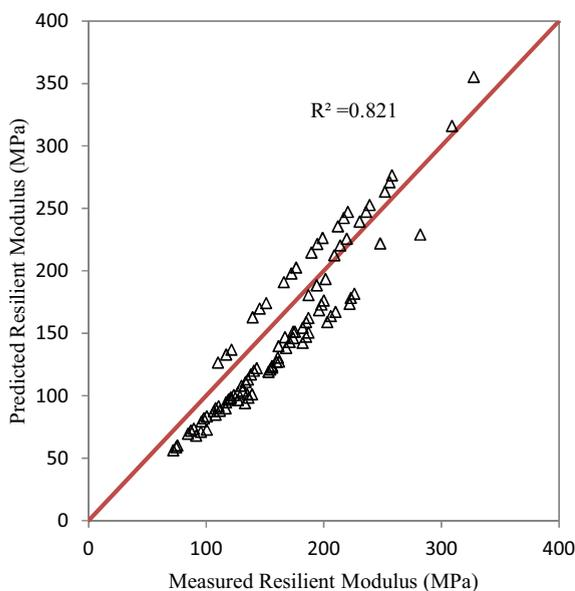
Fig. 6. Measured resilient modulus from tests versus predicted resilient modulus from Eq. (10).
