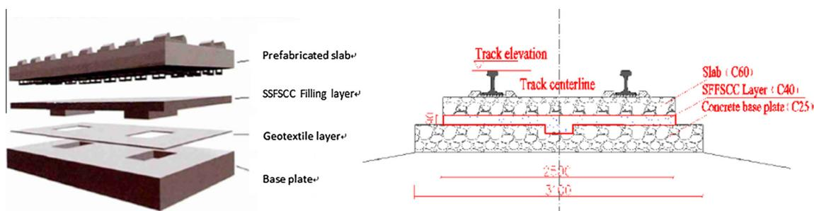
Fig. 1. The structure section and layout of CRTS III slab ballastless track [14,15].
