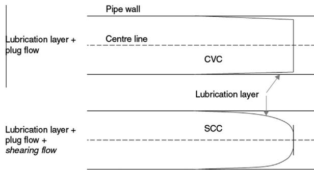
**Fig. 9.** Estimated velocity profile during pumping of conventional vibrated concrete (CVC, top) and self-compacting concrete (SCC, bottom), showing that the bulk SCC is sheared while CVC is not [40].
