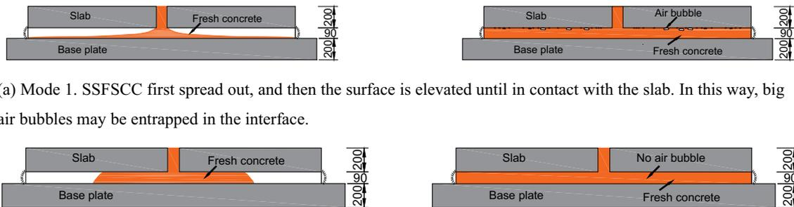
(a) Mode 1. SSFSCC first spread out, and then the surface is elevated until in contact with the slab. In this way, big air bubbles may be entrapped in the interface.
