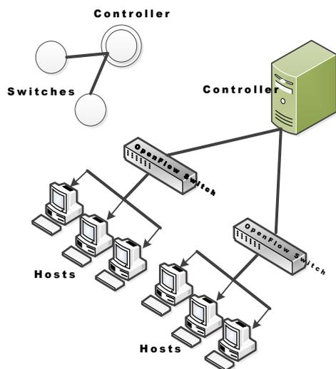
Figure 6(a): Single controller architecture
