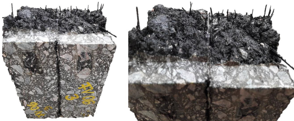
Fig. 12. View of fracture surface after bending tests.
