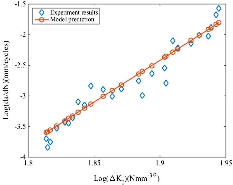
Fig. 10. Variation of crack growth rate ( $da/dN$ ) as a function of stress intensity factor range ( $\Delta K_I$ ) for large specimen [2].
