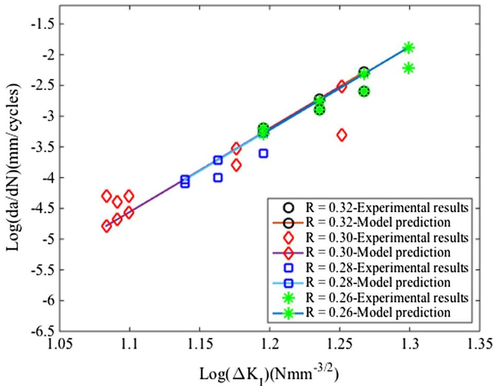
Fig. 11. Variation of crack growth rate ( $da/dN$ ) as a function of stress intensity factor range ( $\Delta K_I$ ) for varying stress ratio [24].
