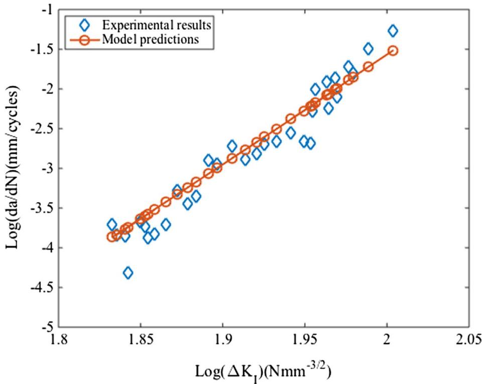
Fig. 9. Variation of crack growth rate ( $da/dN$ ) as a function of stress intensity factor range ( $\Delta K_I$ ) for medium specimen [2].
