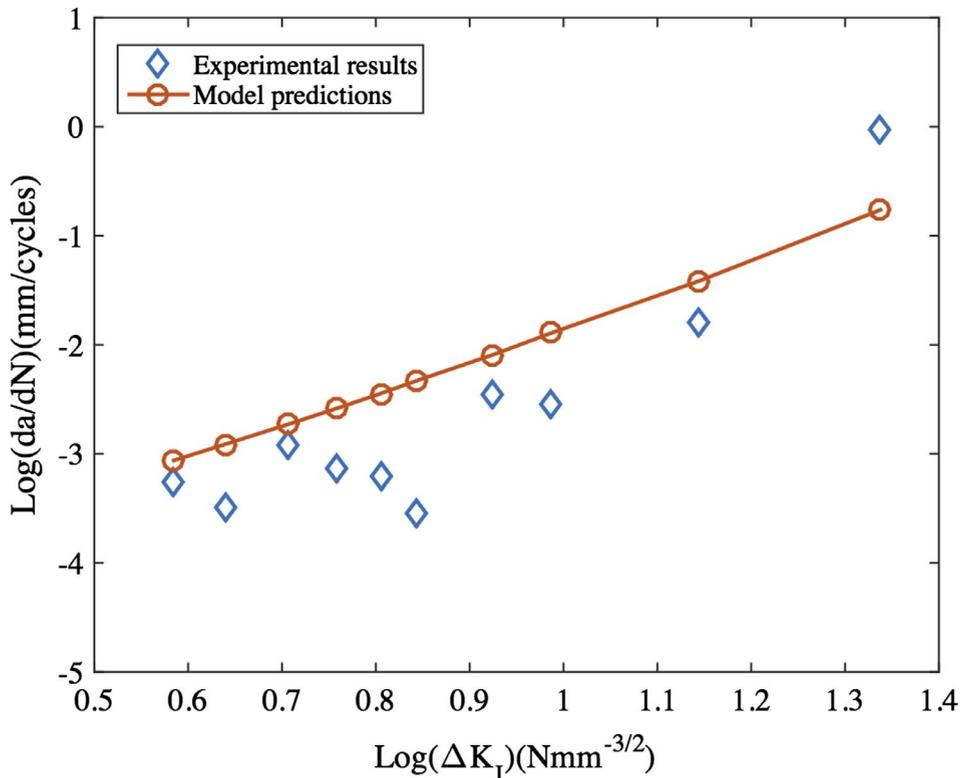
Fig. 5. Variation of crack growth rate ( $da/dN$ ) as a function of stress intensity factor range ( $\Delta K_I$ ) for large specimen [22].
