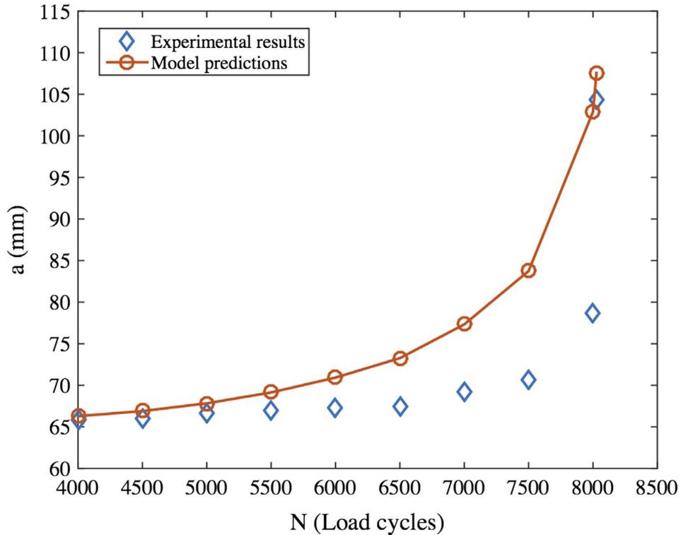
Fig. 7. Variation of crack length ( $a$ ) as a function of number of load cycles ( $N$ ) for large specimen [22].
