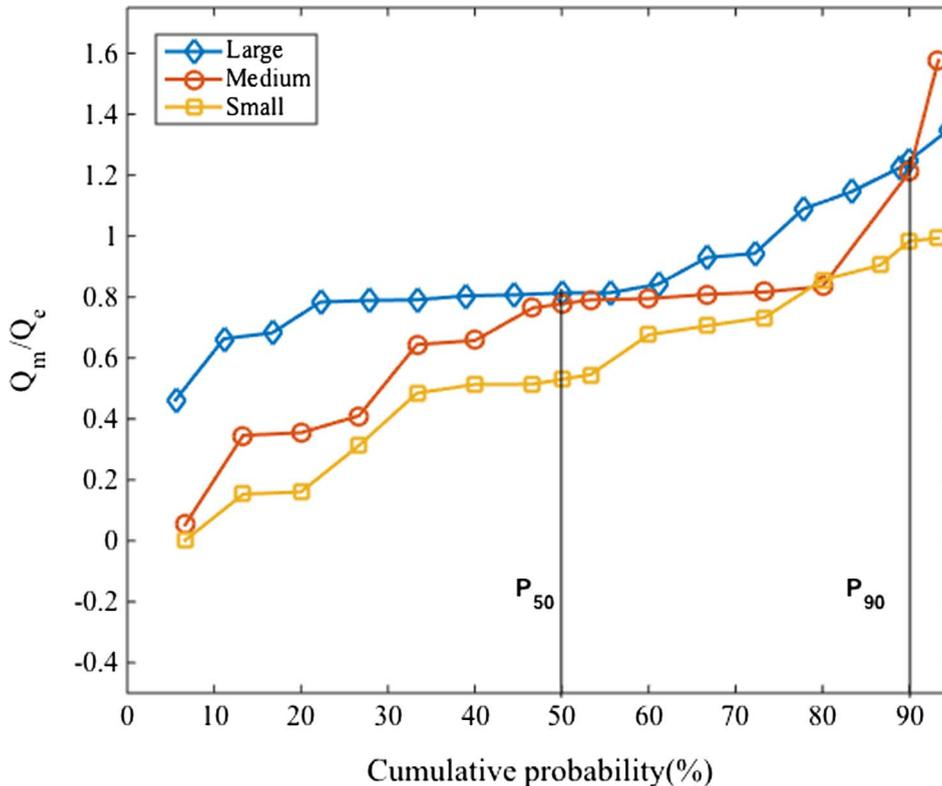
Fig. 12. Cumulative probability plot of ( $Q_m/Q_e$ ) for small, medium and large sized beam specimens [2].
