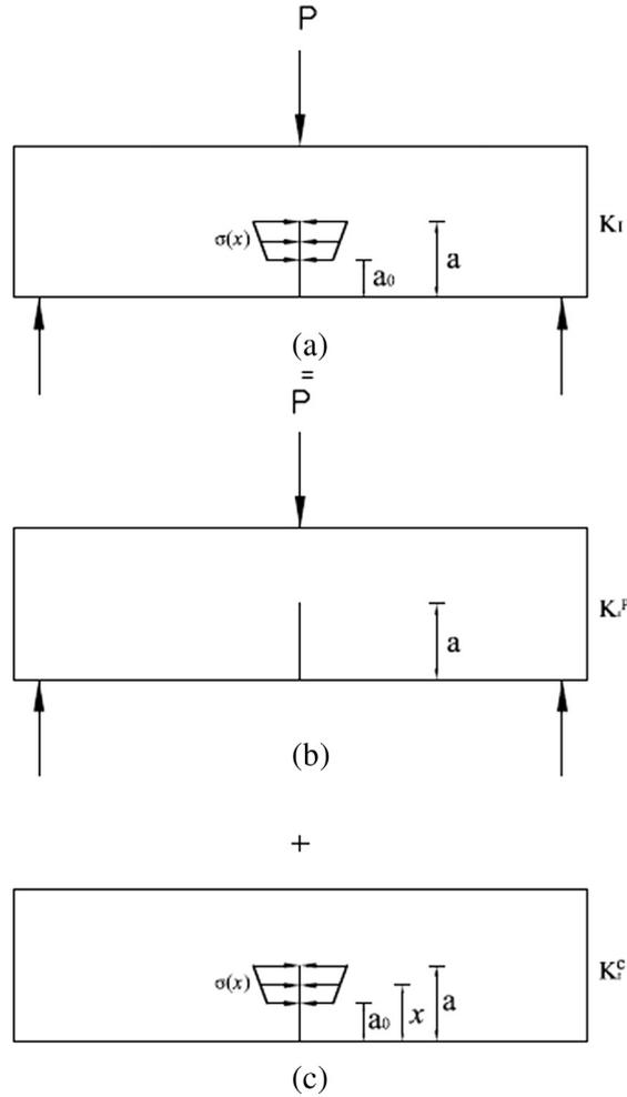
Fig. 15. Superposition of stress intensity factor [25].
