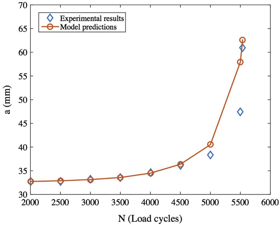
Fig. 6. Variation of crack length ( $a$ ) as a function of number of load cycles ( $N$ ) for medium specimen [22].
