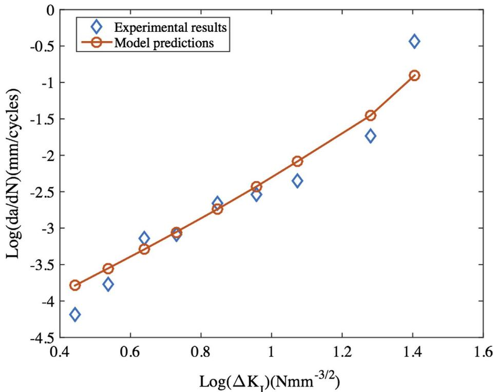
Fig. 4. Variation of crack growth rate ( $da/dN$ ) as a function of stress intensity factor range ( $\Delta K_I$ ) for medium size specimen [22].
