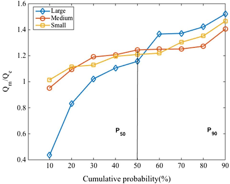
Fig. 13. Cumulative probability plot of ( $Q_m/Q_e$ ) for small, medium and large sized beam specimens [22].
