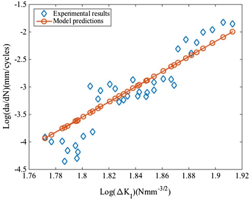
Fig. 8. Variation of crack growth rate ( $da/dN$ ) as a function of stress intensity factor range ( $\Delta K_I$ ) for small specimen [2].
