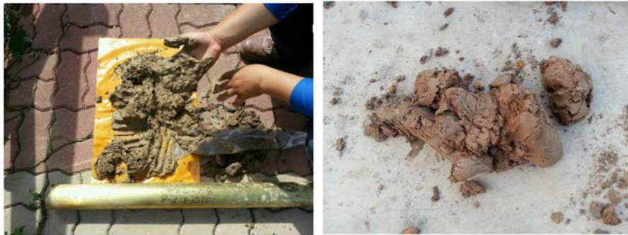
Fig. 6. YC dam: locally deteriorated core samples discovered during geotechnical investigation (2013).
