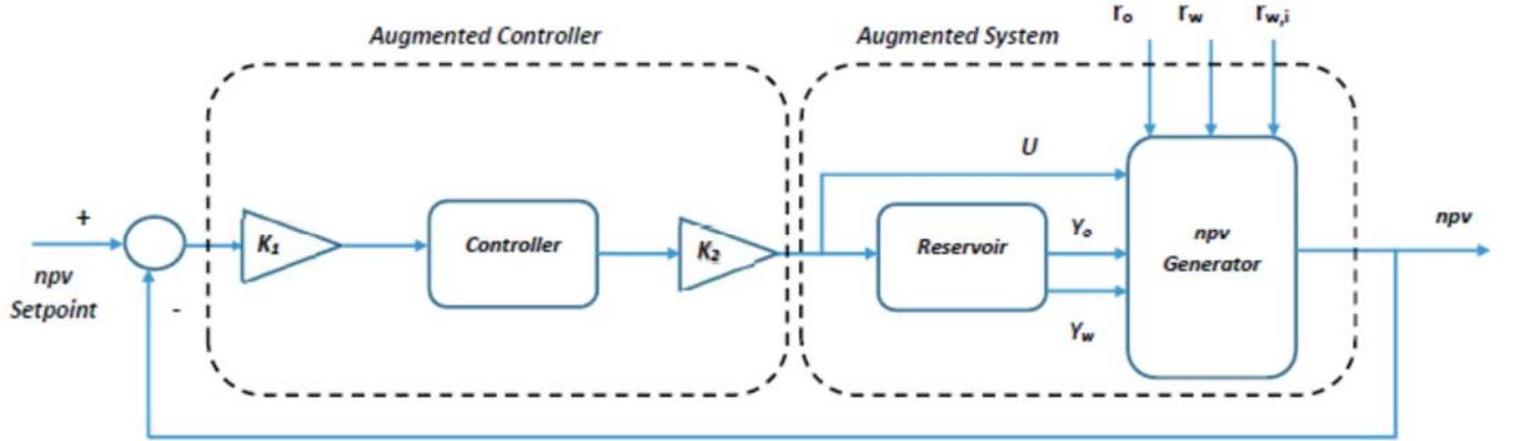
Figure 2. Schematic of the basic closed-loop system for  $npv$  control.
