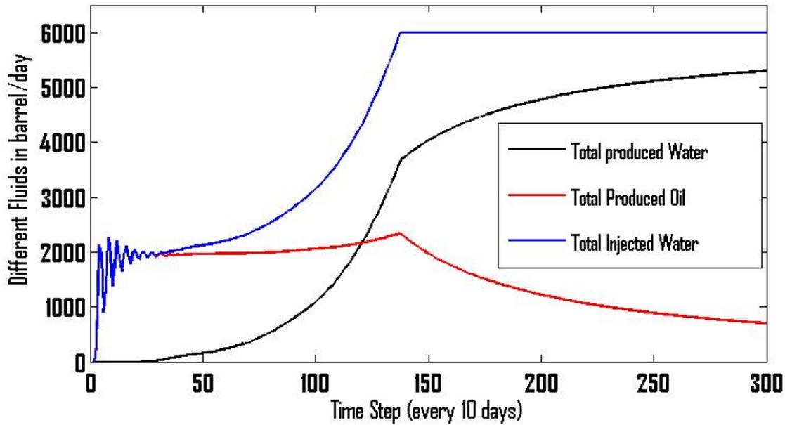
Figure 13. Total oil and water production rates; total injection rate is calculated by the controller
