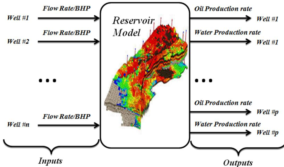
Figure 1. Schematic of oil reservoir model as a controlled system with proper input/output (Hourfar et al., 2016).
