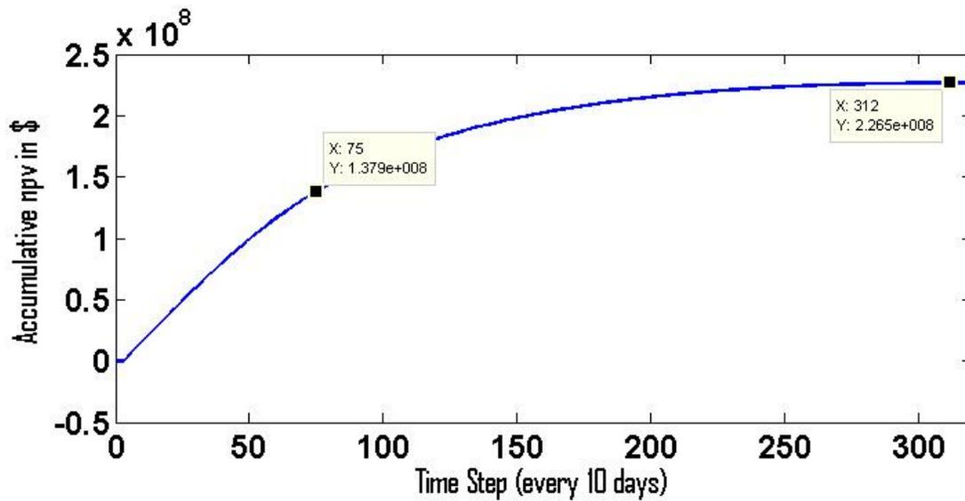
Figure 10. Accumulative *npv*; total injection rate is fixed at 3000 *bbl/day*
