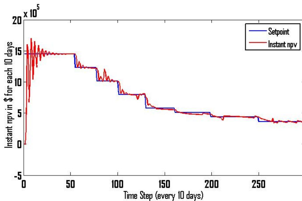
Figure 26. Instant  $npv$ ; controller tries to fix the  $npv$  at the desired setpoint calculated based on AWCI rise as well as considering other effective terms by successfully handling the unexpected cost/price variations
