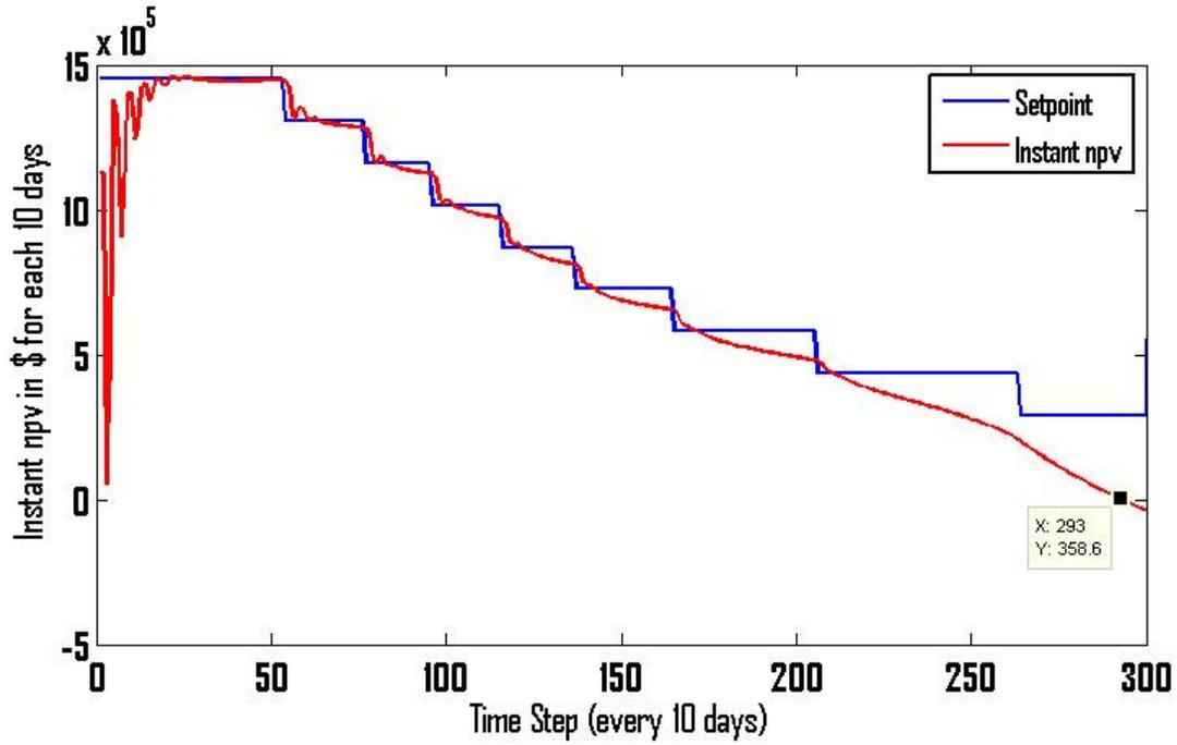
Figure 14. Instant *npv*; controller tries to fix the *npv* at the desired setpoint calculated based on *AWCI* rise
