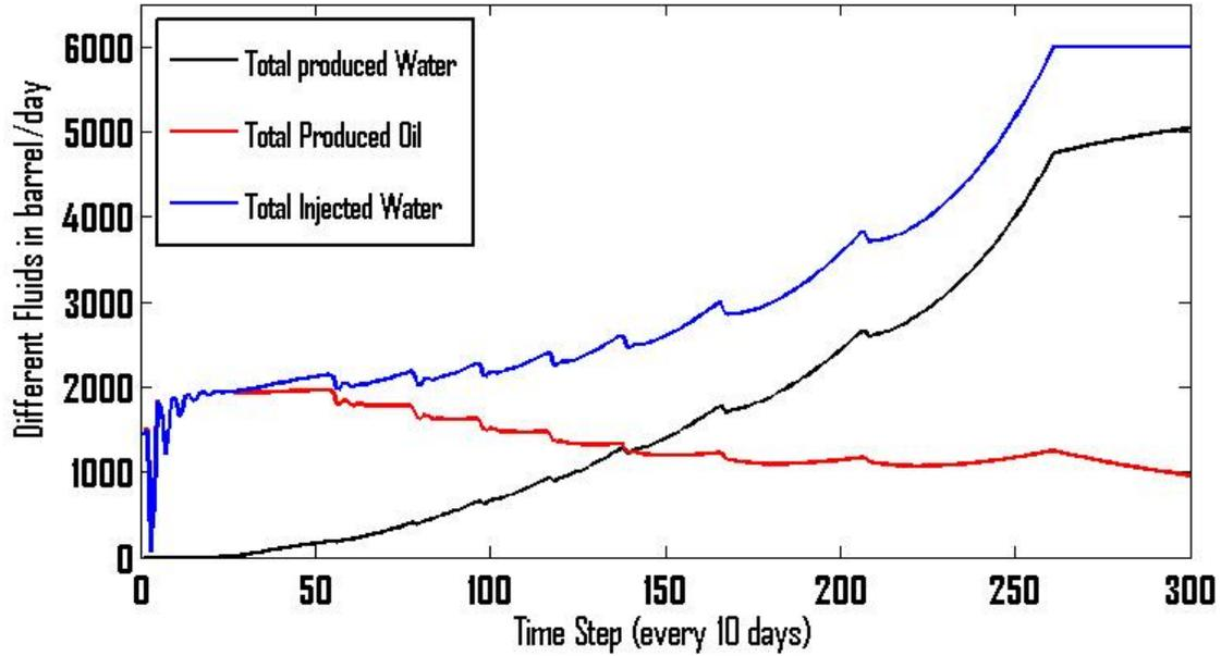
Figure 16. Total oil and water production rates; total injection rate is calculated by the controller
