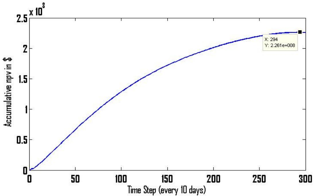
Figure 15. Accumulative  $npv$ ; controller tries to fix the  $npv$  at the desired setpoint calculated based on  $AWCI$  rise
