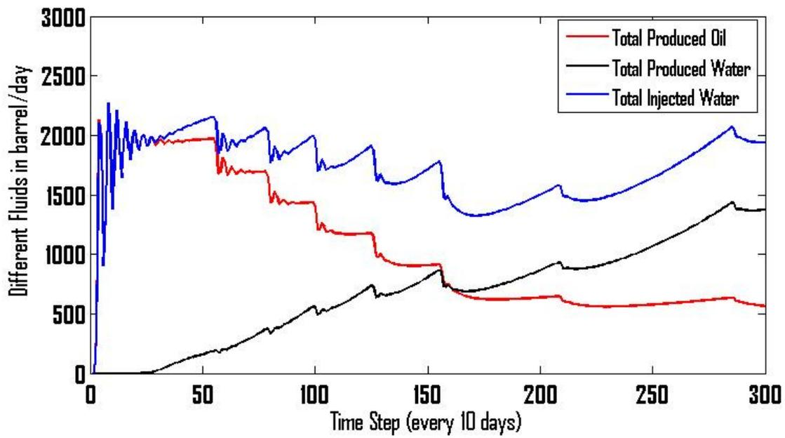
Figure 22. Total oil and water production rates; total injection rate is calculated by the controller
