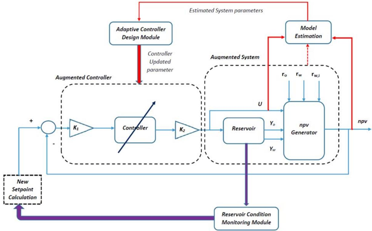
Figure 5. Block-diagram of the modules interconnections in the developed algorithm
