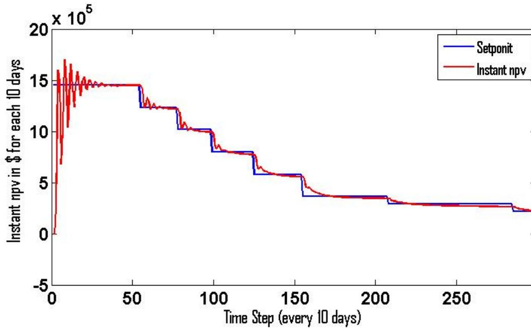
Figure 18. Instant *npv*; controller tries to fix the *npv* at the desired setpoint calculated based on *AWCI* rise as well as considering other effective terms
