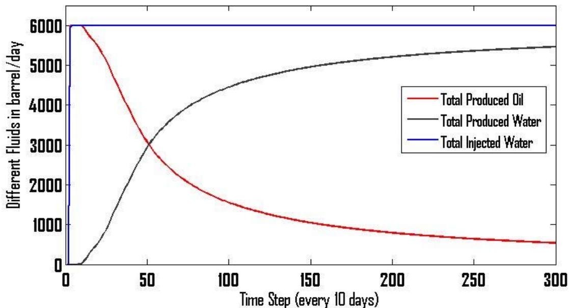
Figure 8. Total oil and water production rates; total injection rate is fixed at 6000 *bbl/day*
