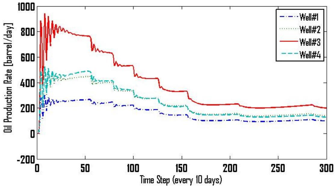
Figure 23. Oil production rates of the producing wells
