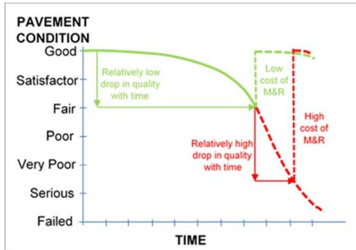
Fig. 1. Illustration of Pavement Condition Variability with Cost of M&R over Time.
