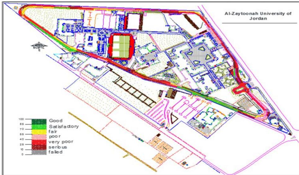
Fig. 6. Road Sections and Sample Units Definitions and Condition Evaluation.
