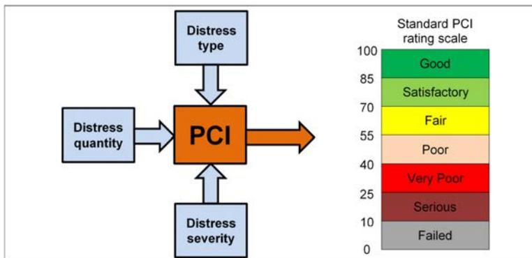
Fig. 3. Rating scale used for Pavement Condition Index (PCI) Method.
