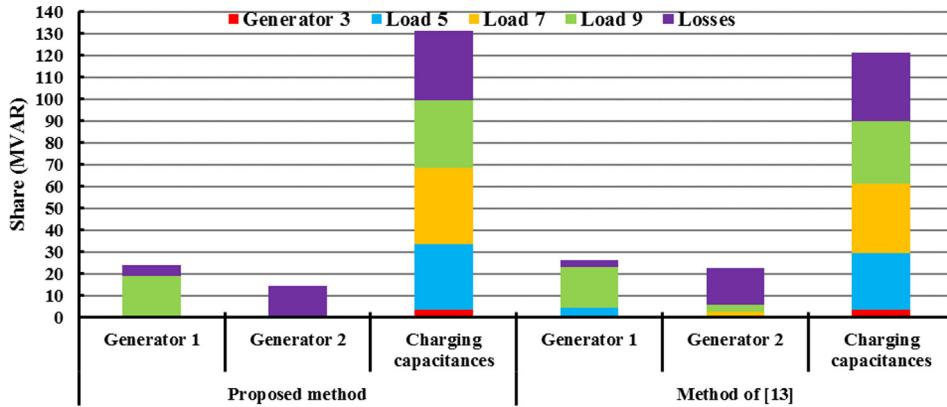
**Fig. 10.** Comparison of two methods for specifying sources' contributions to reactive power consumptions of demands in the IEEE 9-bus system.
