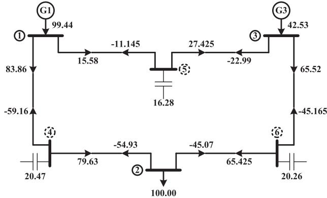
Fig. 4. One-line diagram of the modified 3-bus system with reactive power flows (MVAR).
