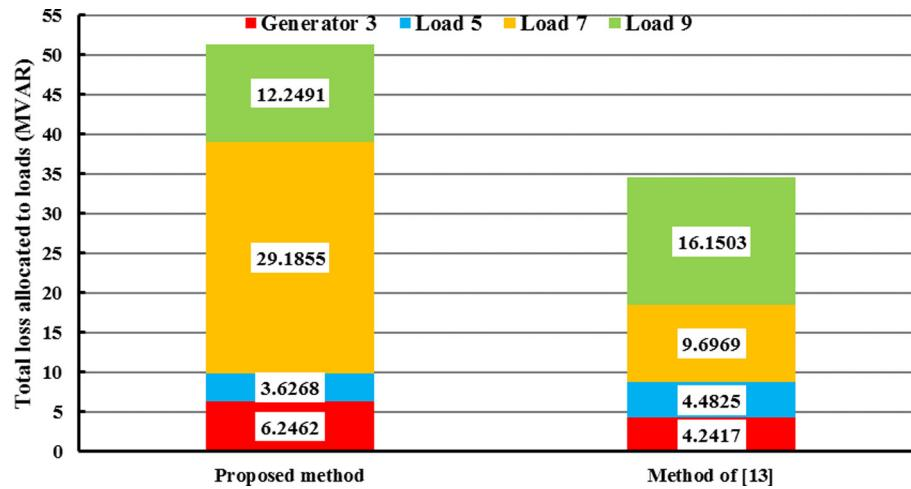
**Fig. 11.** Comparison of two methods for allocating total reactive losses to loads in the IEEE 9-bus system.
