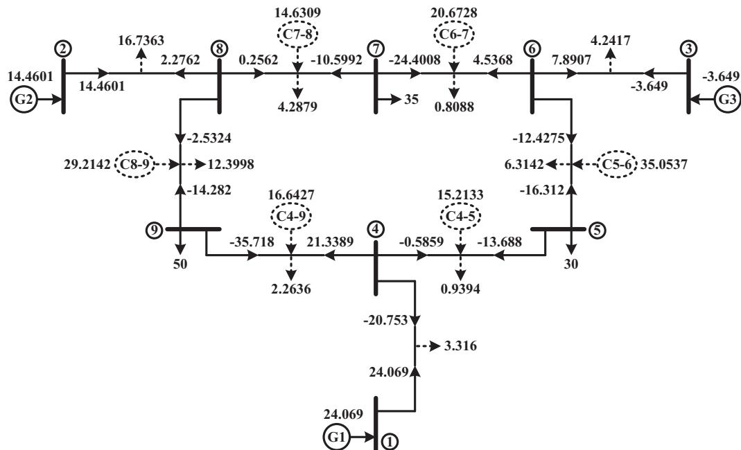
Fig. 8. One-line diagram of the IEEE 9-bus system with reactive power flows (MVAR).
