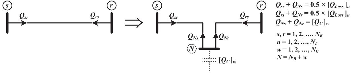
**Fig. 1.** Representation of equivalent model for generating branch.
