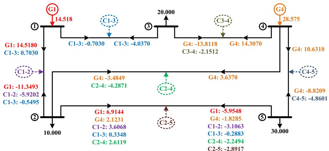
Fig. 9. Sources' contributions to reactive power flows of branches in the 5-bus system (MVAR).
