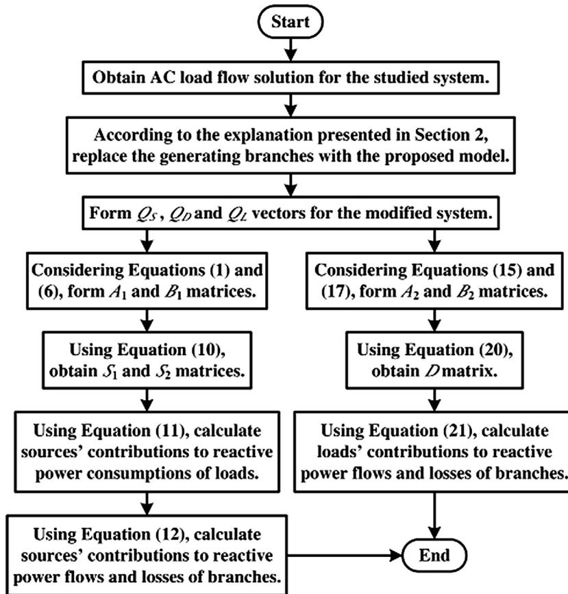
Fig. 2. Flowchart of the proposed method for reactive power tracing.
