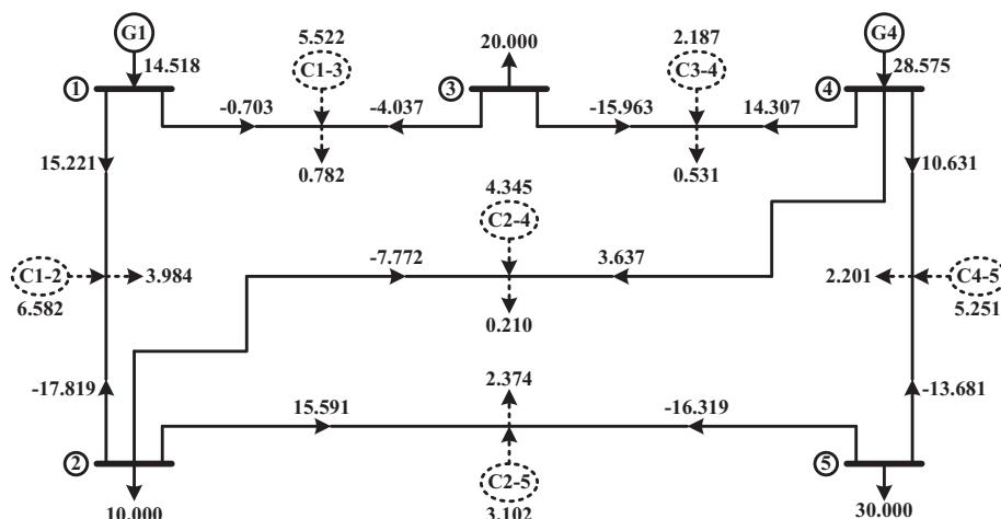
**Fig. 7.** One-line diagram of the 5-bus system with reactive power flows (MVAR).
