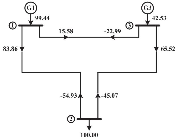
Fig. 3. One-line diagram of the 3-bus system with reactive power flows (MVAR).
