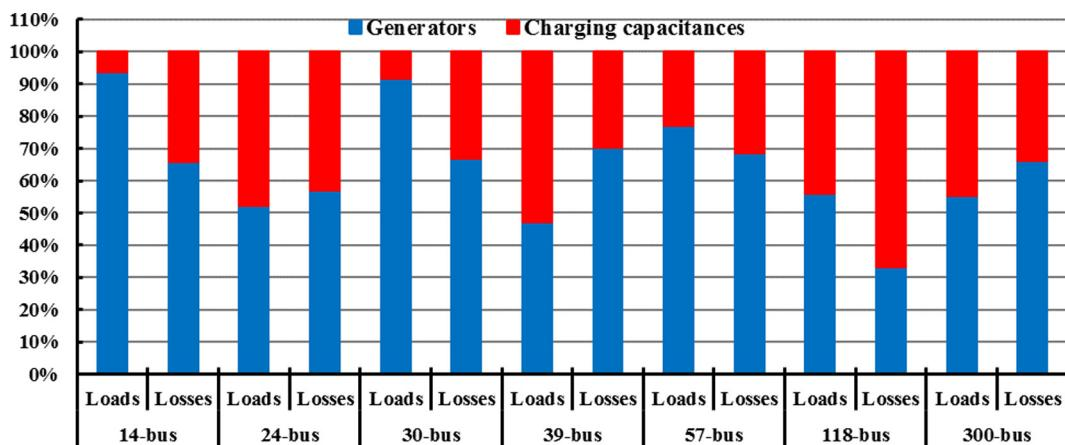
**Fig. 6.** Sources' contributions to total reactive loads and losses of IEEE standard systems.
