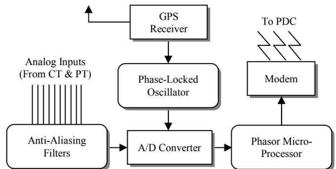
Fig. 1. Basic components of Phasor Measurement Unit
