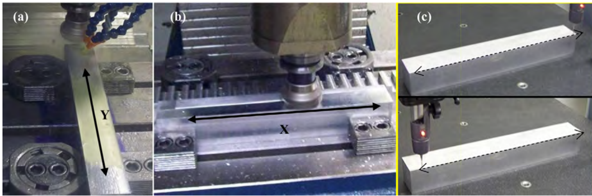
Fig. 5. (a) Milling along the X-axis; (b) milling along the Y-axis; (c) MMC 3D measurement.
