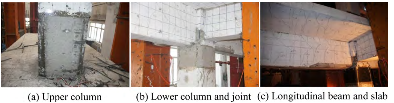
Fig. 8. Failure modes of specimen SC.
