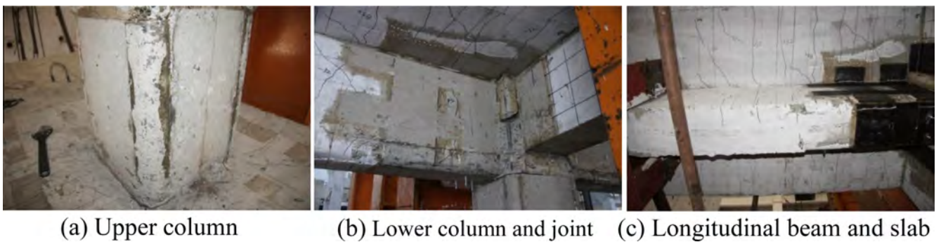
Fig. 9. Failure modes of specimen SCBU.
