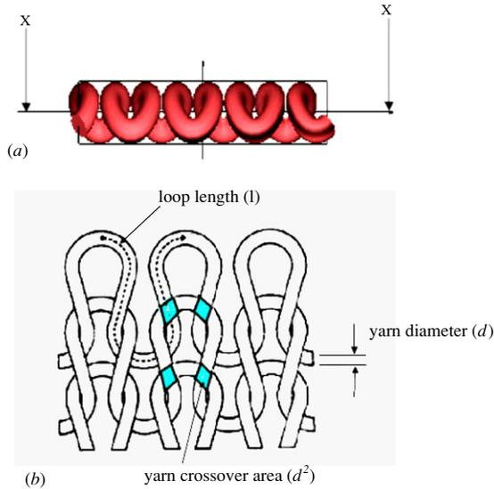
**Figure 3.** Sectional views of plain knitted fabric: (a) cross-section view; (b) view in the  $XX$  plane.
