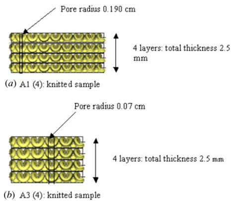
**Figure 7.** Simulated cross sectional representation of the knitted fabric samples used for the test.
