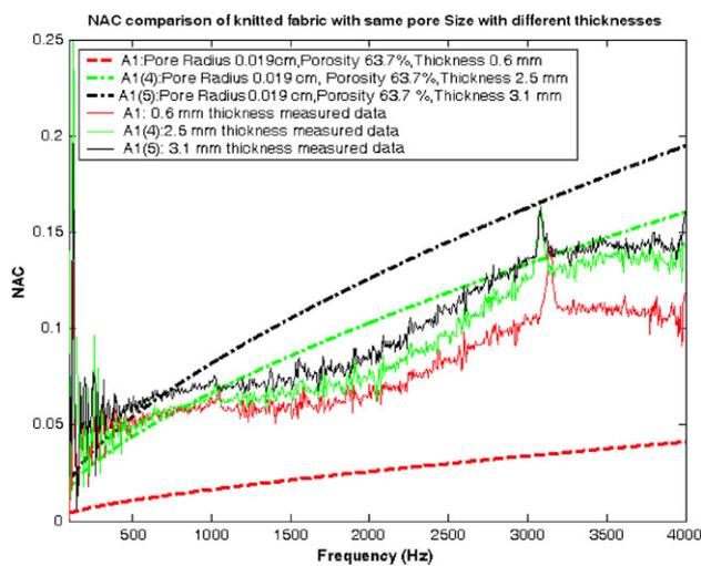
**Figure 8.** NAC data for different thicknesses of plain structure A1.
