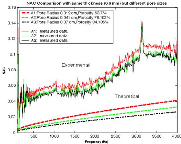
**Figure 5.** NAC for plain knitted structures with the same thickness but different pore sizes.
