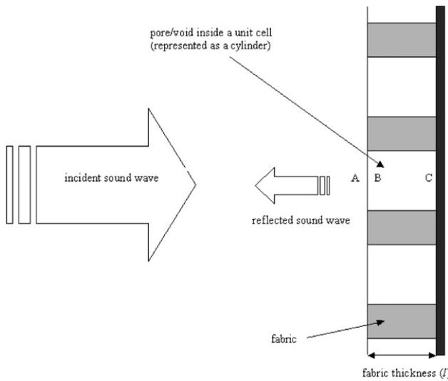
Figure 2. Sound absorption by a pore formed by the void of a unit cell, which is backed by a rigid wall.
