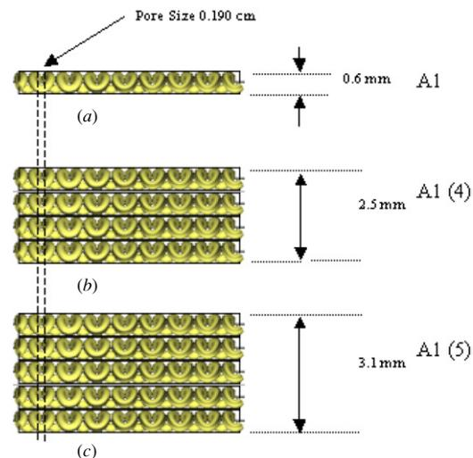
**Figure 9.** Simulated cross-sectional representation of the knitted samples of A1 fabric used for the test: (a) single layer of 0.6 mm thickness; (b) four layers with a total of 2.5 mm thickness; (c) five layers with a total of 3.1 mm thickness.
