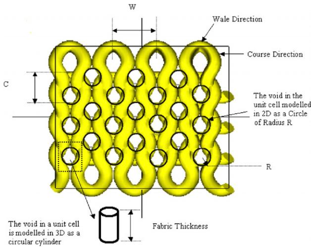
Figure 1. Technical face of a plain knitted structure.
