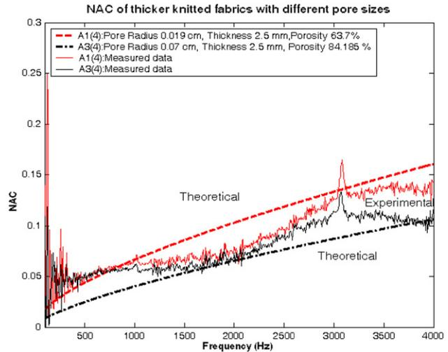
**Figure 6.** NAC of two knitted fabrics with different pore sizes with each fabric sample comprising four layers giving a total thickness of 2.5 mm.
