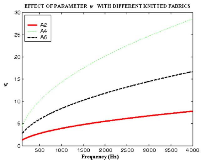
**Figure 4.** The variation of the dimensionless parameter  $\psi$  with the pore radius and frequency.
