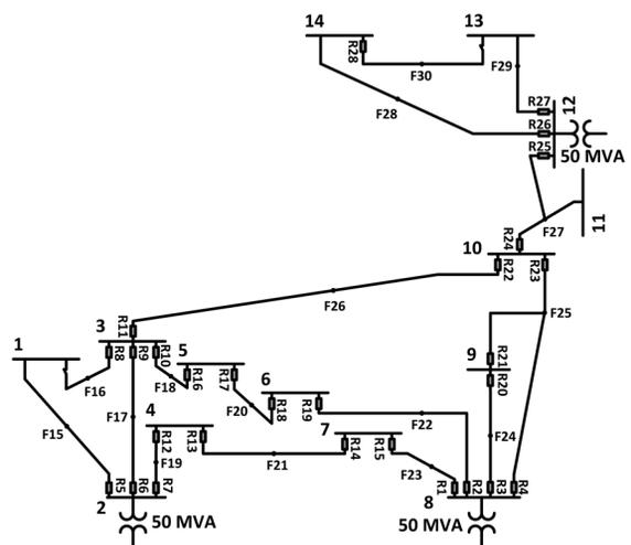
Fig. 4. Power distribution system of the IEEE 30-bus system under study.
