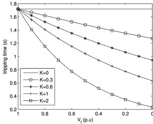
Fig. 2. Effect of the setting  $K$  on the proposed relay tripping time with  $M = 1.5$  and  $TDS = 0.1$ .
