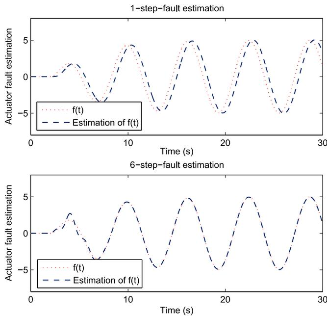
Fig. 4. Response curves of  $f(t)$  and its estimates for  $a = 5, b = 0$ .
