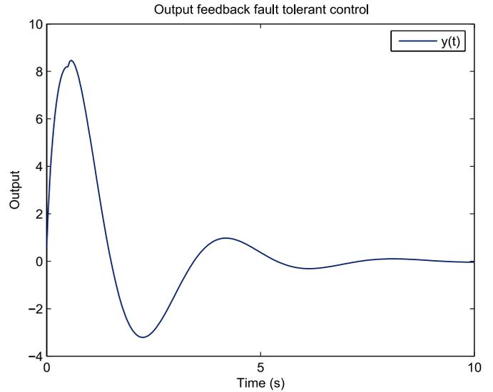
Fig. 11. Response curve of output  $y(t)$  under initial condition  $\phi(t) = [0.5\pi \ 0.75\pi \ -5]^T$ .
