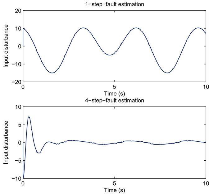
Fig. 9. Response curves of input disturbance from  $\dot{f}(t)$  and  $\dot{f}(t) - \dot{\hat{f}}_3(t)$ , respectively.
