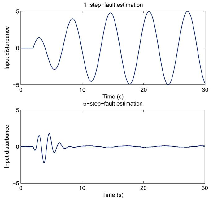
Fig. 6. Response curves of input disturbances  $\hat{f}(t)$  and  $\hat{f}(t) - \hat{f}_5(t)$  by one and six-step fault estimation for  $a = 5, b = 0$ , respectively.
