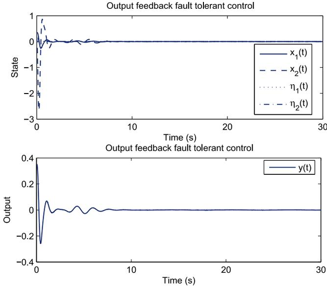
Fig. 7. Response curves of state and output  $y(t)$  under initial condition  $\phi(t) = [\pi/3 \ 0]^T$  for  $a = 5, b = 0$ .
