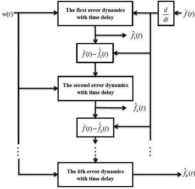
Fig. 1. Flowchart of  $k$ -step fault-estimation.
