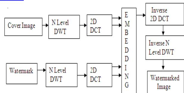
Figure: 4 Generalized DWT –DCT based Watermarking
