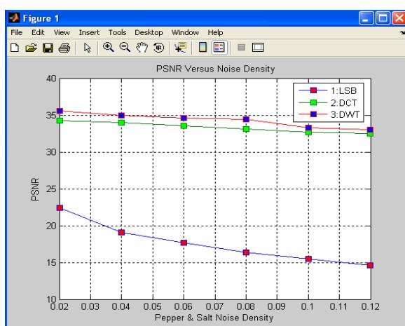
**Figure: 6 Comparative plotting of PSNR Versus Noise Density for LSB, DCT and DWT based watermarking**
