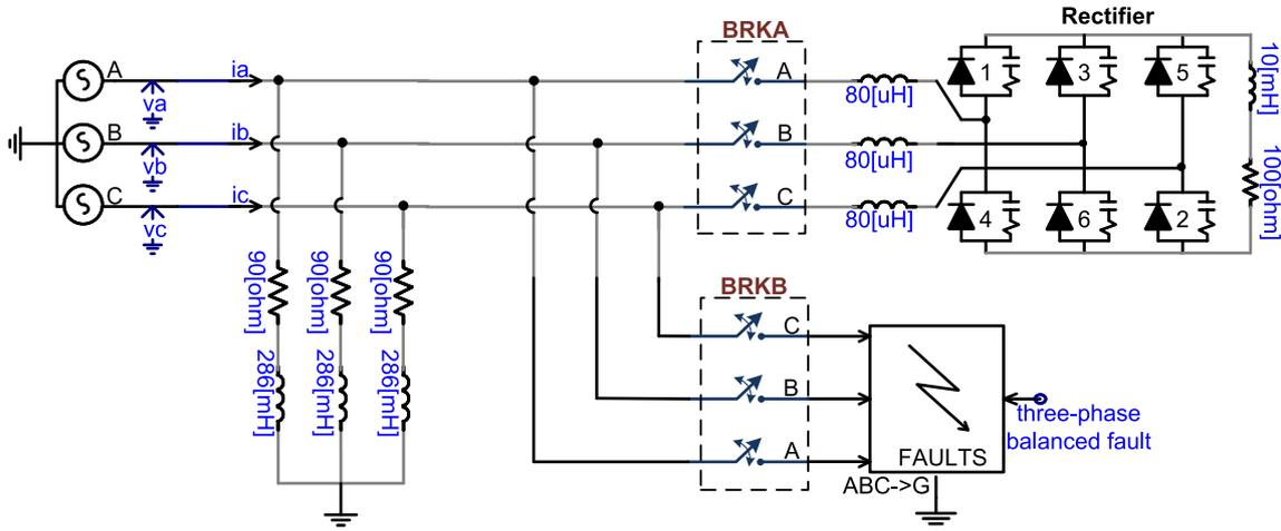
Fig. 3. Power circuit of the simulation test system.
