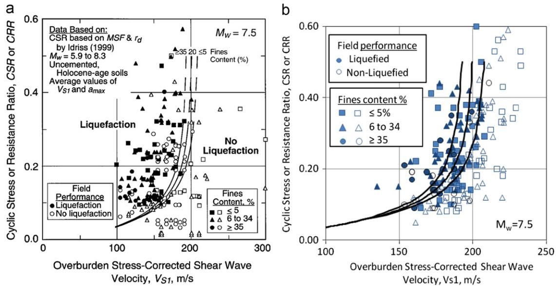
Fig. 6. CRR- $V_{s1}$  curves for different fines content and evaluation of proposed  $V_s$  equation for conversion of SPT resistance to shear wave velocity, (a) Andrus and Stokoe (2000)'s  $V_s$  database, (b) Cetin (2000)'s SPT database.
