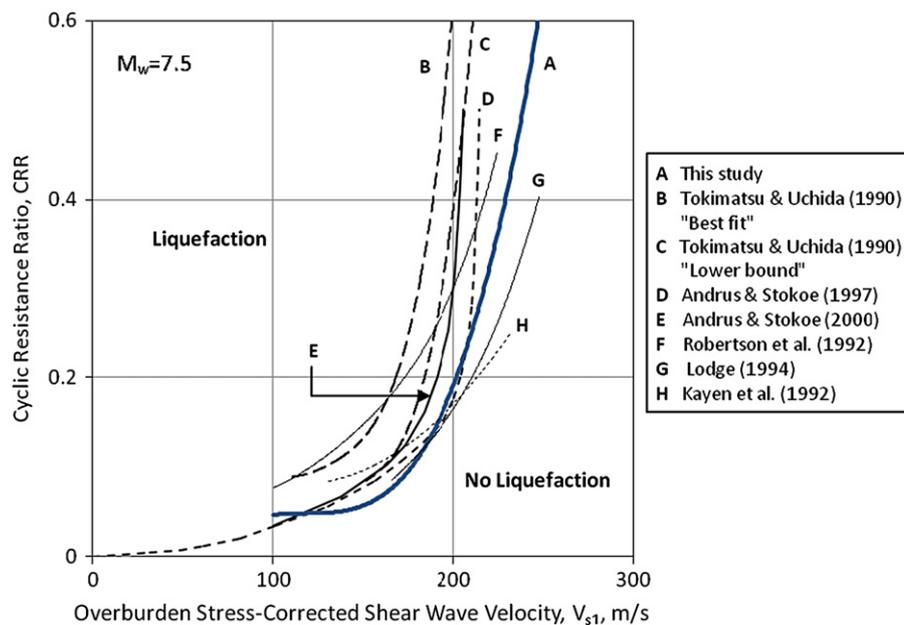
Fig. 5. Comparison of available  $V_{s1}$ -CRR correlations and correlation derived by new  $V_s$  equation developed in this study.
