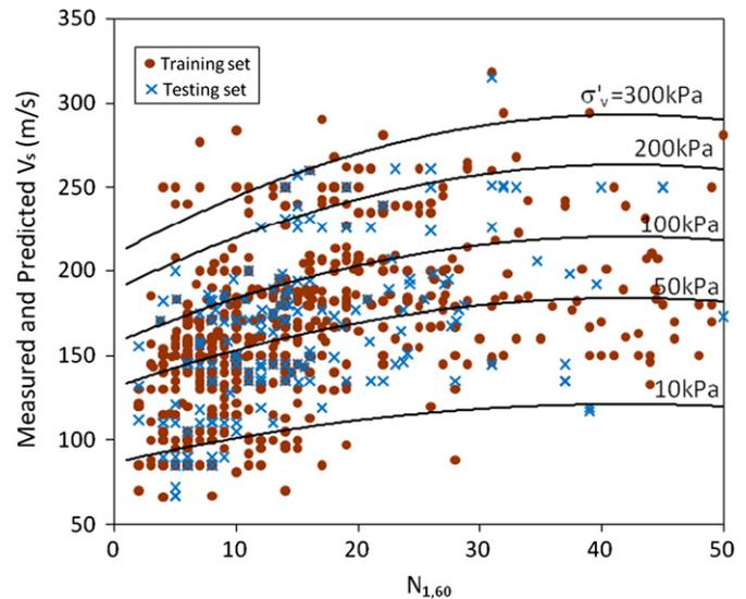
Fig. 3. Parametric study of the developed equation (curves) and measured values (data points).
