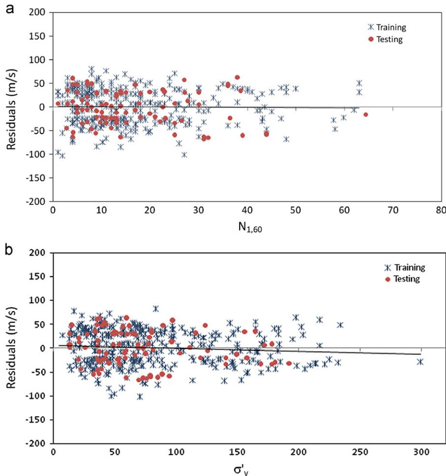
Fig. 2. Residuals of training and testing sets versus (a) corrected SPT blow counts, and (b) effective overburden pressure.
