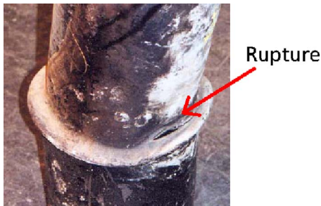
Fig. 3 Shape of the wrinkle in the field NPS10 line pipe
