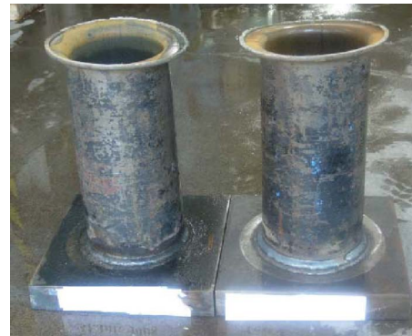
Fig. 13 Specimen 3 split into two pieces during the pressure test
