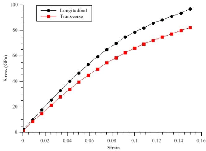
Fig.4. Stress-Strain curves of GS along the longitudinal and the transverse direction
