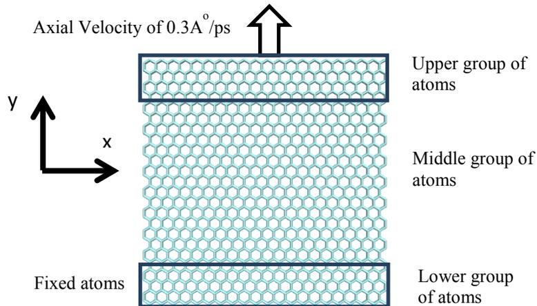
Fig.3. Schematic illustration of the tension test on GS along the longitudinal direction
