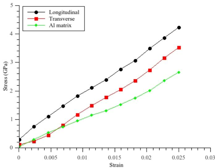
Fig.5. Stress-Strain curves of Al and GS-Al nanocomposite along longitudinal and transverse direction
