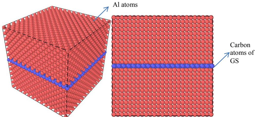
Fig. 1. RVE containing single layer GS in Al matrix
