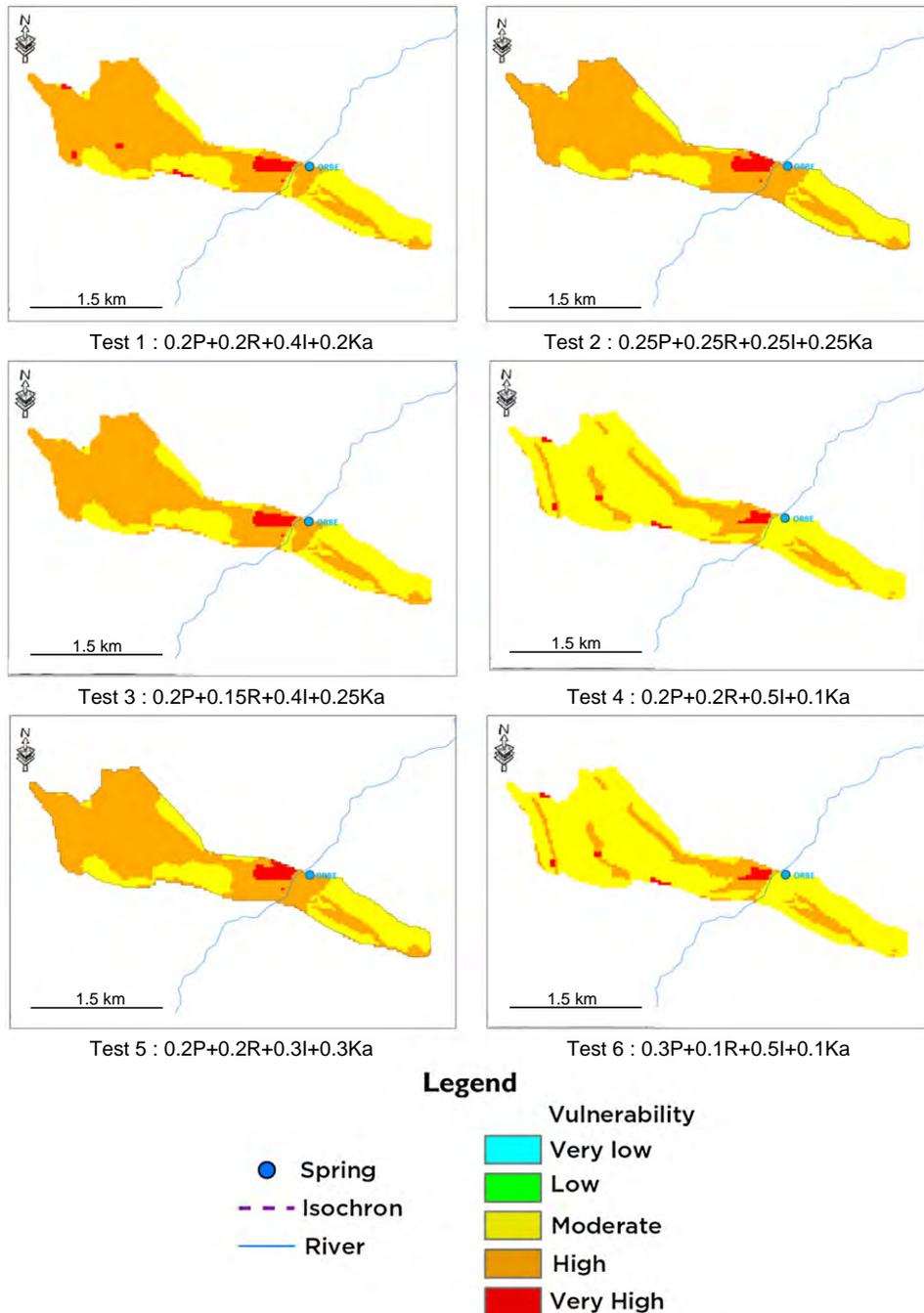
Fig. 8. Intrinsic vulnerability map for the resource of the Orbe spring.
