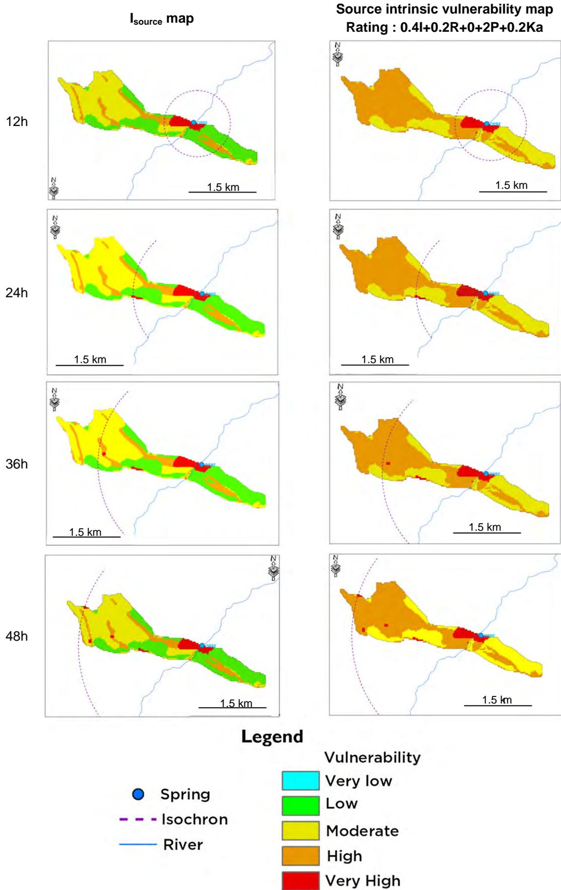
Fig. 9. I<sub>source</sub> maps and the corresponding source-vulnerability maps for the 4 isochrones (12, 24, 36, 48 h) considered by PaPRIKa methodology.
