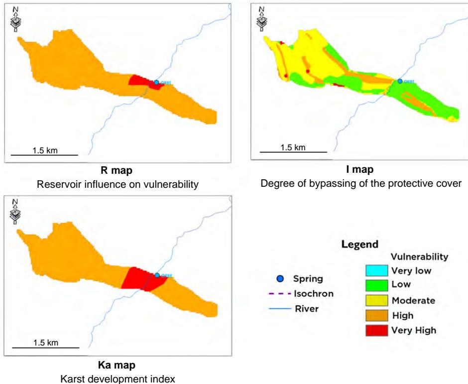
Fig. 7. R, I, Ka maps characterizing the intrinsic vulnerability of the Orbe karst system.
