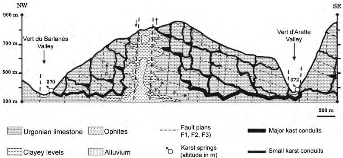
Fig. 2. Schematic cross section through the Orbe Spring aquifer system, modified from Rey (2007).
