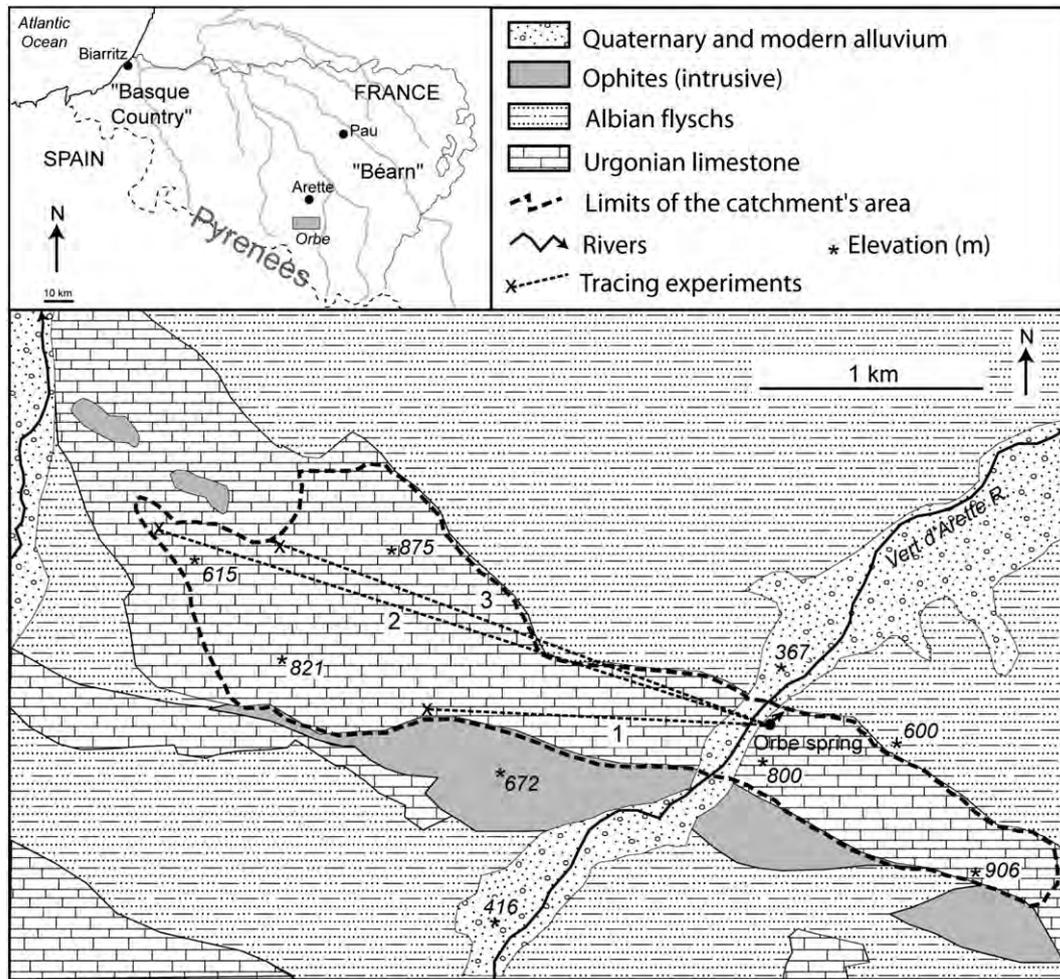
Fig. 1. Location of the spring and simplified geological map of the study area. The numbering of the tracing experiments refers to Table 5.
