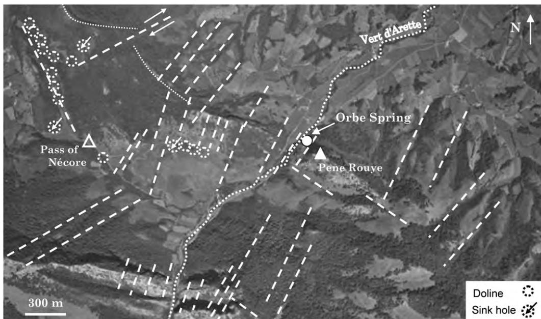
Fig. 3. Map of the karstic features and lineaments recognized on the Orbe catchment area, modified from Rey (2007).
