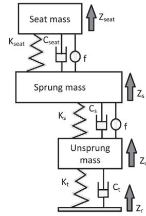
(a) Model of one corner of vehicle with seat
