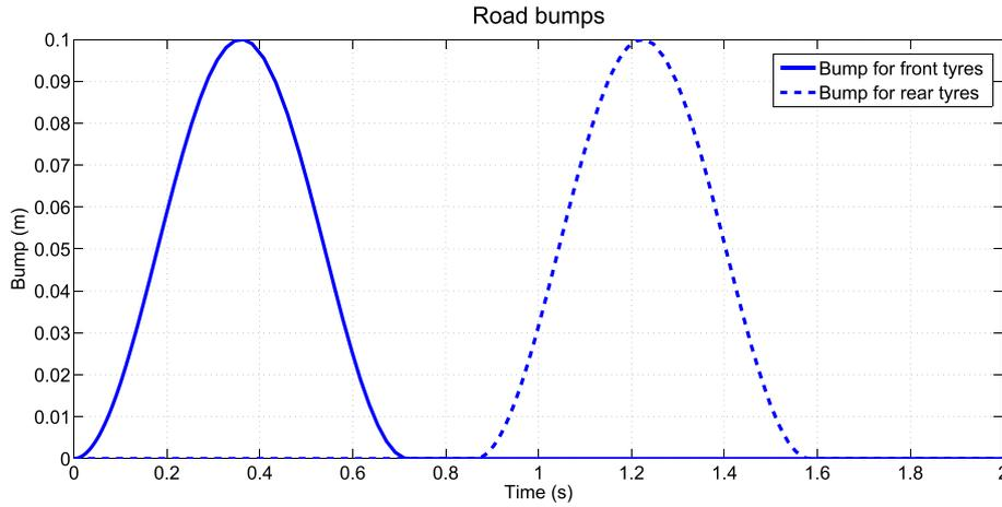
Fig. 2 Road disturbance for vehicle.
