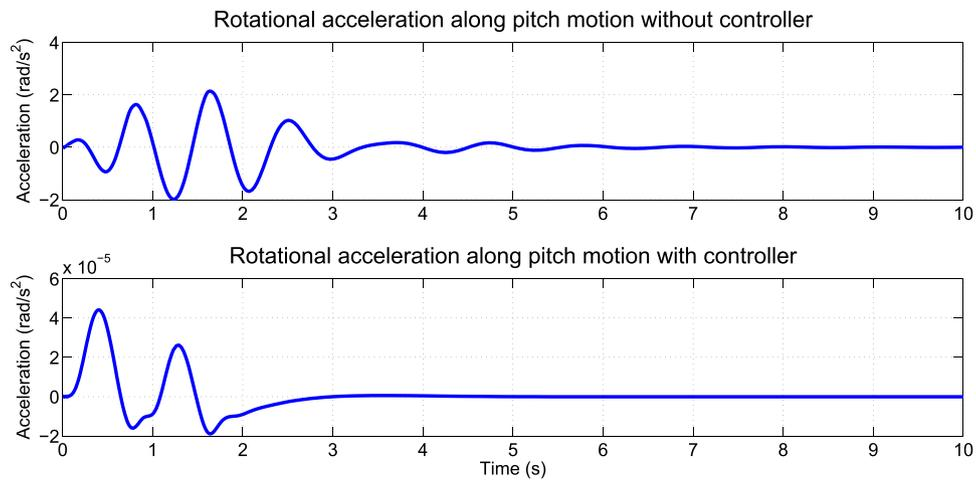
(b) Rotational acceleration of vehicle along pitch motion
