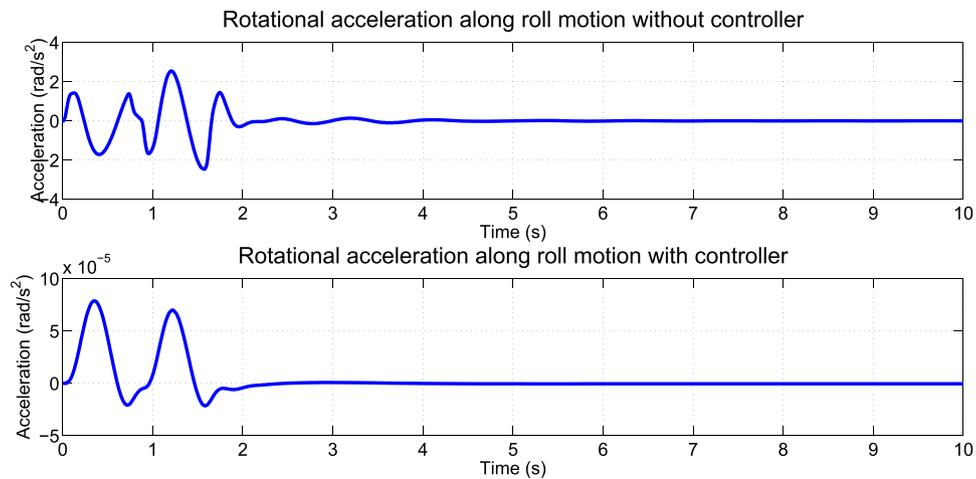
(c) Rotational acceleration of vehicle along roll motion
