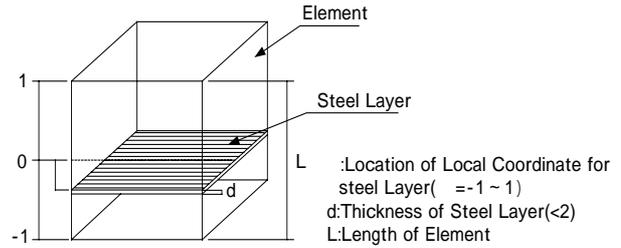
Figure 5 Local coordinate and location of steel layer
