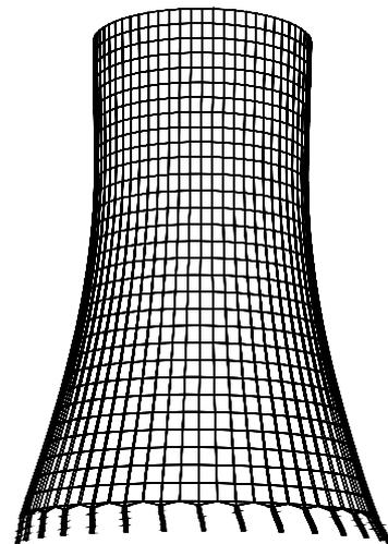
Figure 9 Deformation under Step Load (I-column)
