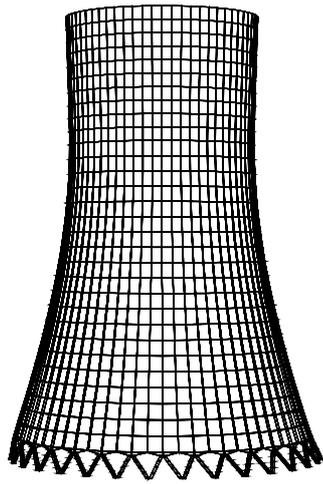
Figure 10 Deformation under Step Load
