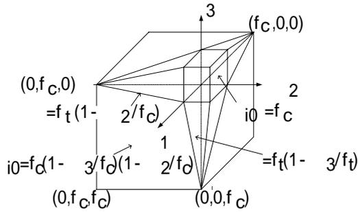
Figure 3 Crack condition
