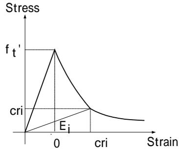
Figure 4 Concrete in Tension
