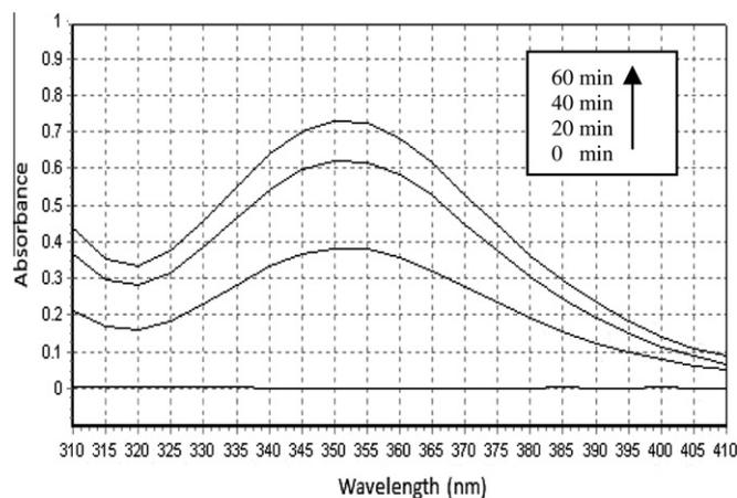
**Fig. 3.** Temporal evolution of absorption spectra for iodide dosimeter under sonication (1 MHz, 2 W/cm<sup>2</sup>). The maximum absorption is related to 60 min sonication.
