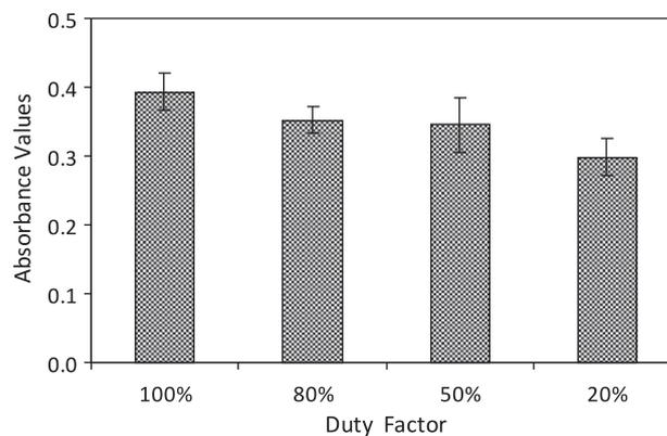
**Fig. 6.** Mean  $\pm$  SD of the absorbance value by 1 MHz pulsed irradiation with compensated sonication duration at different duty cycles ( $I = 2$  W/cm<sup>2</sup>). Values obtained from 5 independent experiments (CV = 5–11%).
