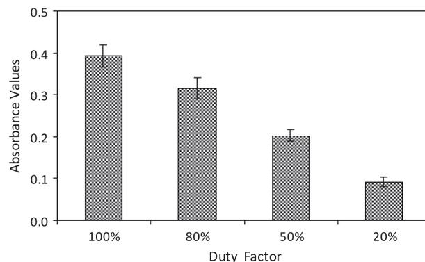
**Fig. 5.** Mean  $\pm$  SD of the absorbance by 1 MHz irradiation at different duty cycles ( $I_{SATA} = 2$  W/cm<sup>2</sup> and sonication duration 20 min). The absorbance values were recorded based on 5 independent runs (CV = 6–12%).
