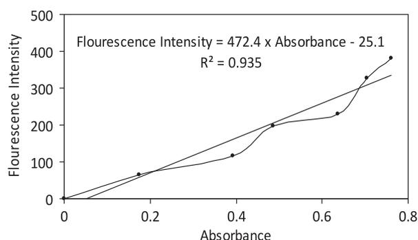
**Fig. 10.** Pearson correlation and linear regression analyses between absorbance and fluorescence intensity (count) at different sonication duration with constant intensity (2 W/cm<sup>2</sup>).
