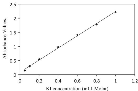
Fig. 1. Calibration curve for KI solution with different concentration.
