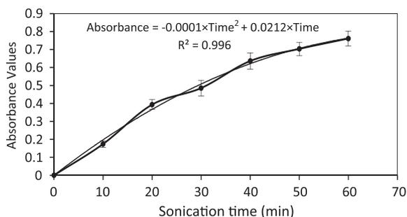
**Fig. 2.** Absorbance values (CV = 5–10%) due to sonication duration (min) for the continuous mode in 1 MHz ultrasound irradiation. Error bars show the standard deviation of mean values obtained from 5 independent experiments.
