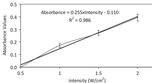
**Fig. 4.** Dependence of absorbance value on sonication intensity (0.5–2.0 W/cm<sup>2</sup>) for the continuous mode of ultrasound irradiation (CV = 6–10%). Error bars show the standard deviation of mean values obtained from 5 independent experiments.
