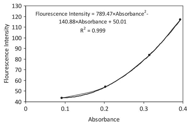
**Fig. 9.** Correlation and polynomial regression analyses between absorbance and fluorescence intensity (count) at different duty cycles with constant intensity (2 W/cm<sup>2</sup>) and 20 min sonication.
