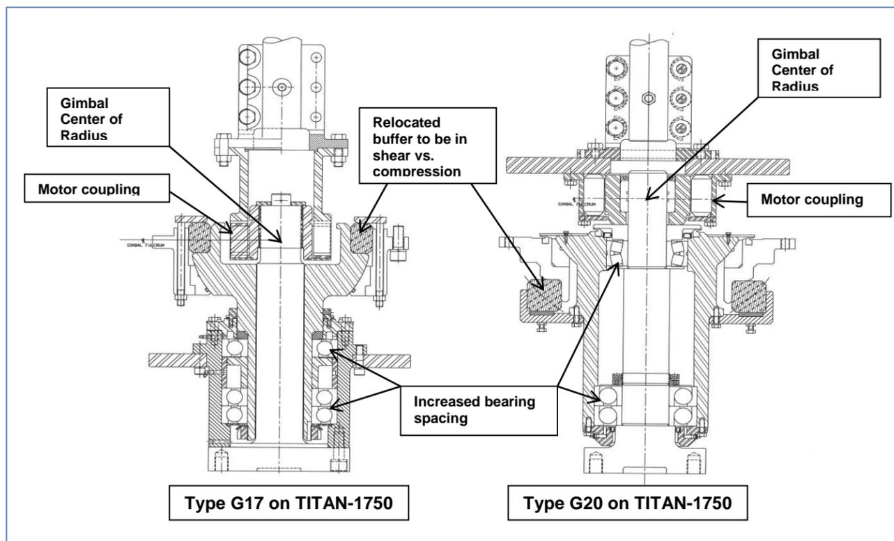
Figure 4: Comparison of G17 and G20 head designs
