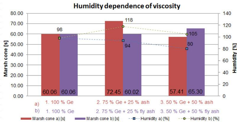
Fig. 1. Humidity dependence of viscosity suspension based on Ge clay, ash and fly ash.
