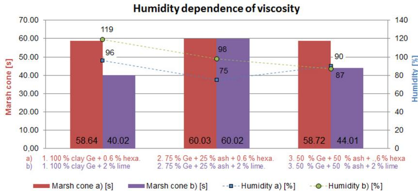
Fig. 3. Humidity dependence of viscosity suspension based on Ge clay, ash, pl. additives and lime.
