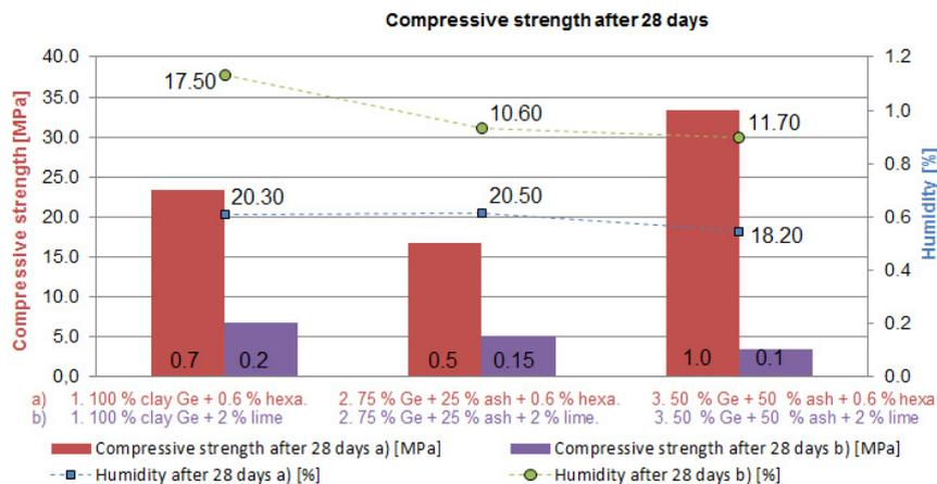
Fig. 4. Results of the strength determination and humidity of samples based on Ge clay, ash, pl. additives and lime.
