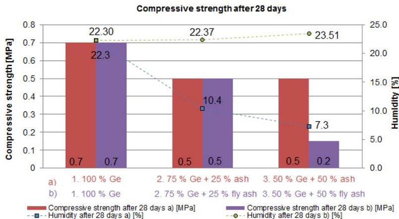
Fig. 2. Results of the strength determination and humidity of samples based on Ge clay, ash and fly ash.
