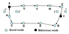
Figure: 1 Wormhole through packet encapsulation
