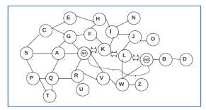
Out-of-band channel normal channel In band channel malicious node Figure 3: wormhole attack
