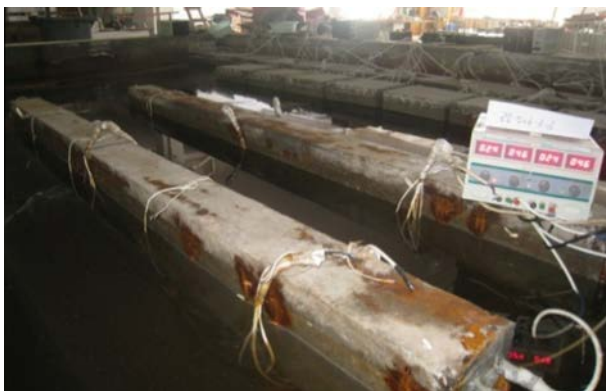
Fig. 2. Accelerated corrosion of prestressed concrete beams.
