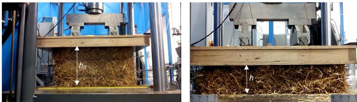
**Fig. 4.** The compression device and the two different configurations. (left) edge, at the beginning of a test; (right) flat, with a strain of 0.77.
