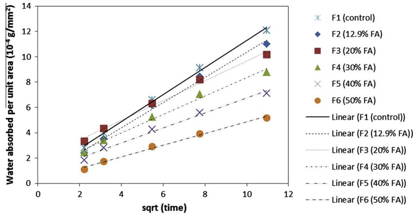
Fig. 4. Surface water absorption against time<sup>1/2</sup> for F-series specimens.
