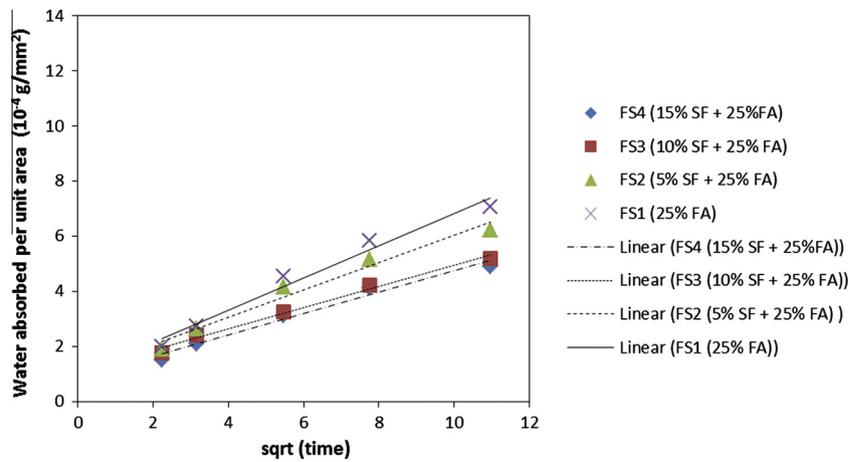
Fig. 5. Surface water absorption against time<sup>1/2</sup> for FS-series specimens.
