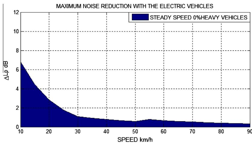
Fig. 8. Variation of noise levels between 100% AVAS-EV vs 100% ICEV traffic flows, with no heavy vehicles.
