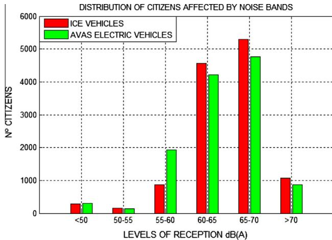
Fig. 12. Difference of simulation of traffic flow of AVAS vs ICE vehicles.
