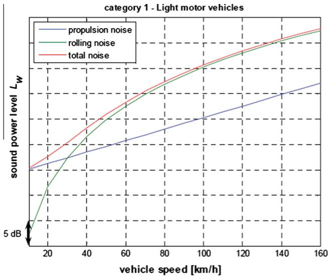
Fig. 3. Contribution of different sub-sources to the total sound emitted by a vehicle [5].
