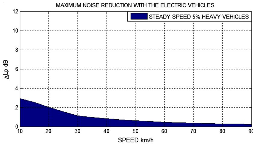
Fig. 7. Variation of noise levels between 95% Light EV vs 95% Light ICEV, plus 5% ICE heavy vehicles of the total.
