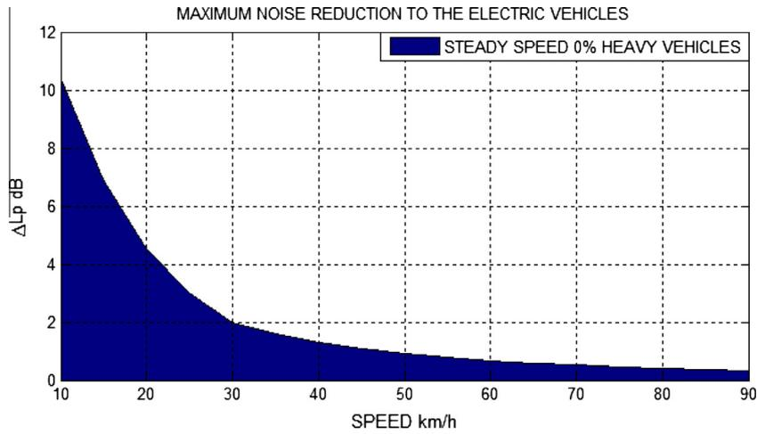
Fig. 6. Variation of noise levels between 100% EV vs 100% ICEV traffic flows, no heavy vehicles.
