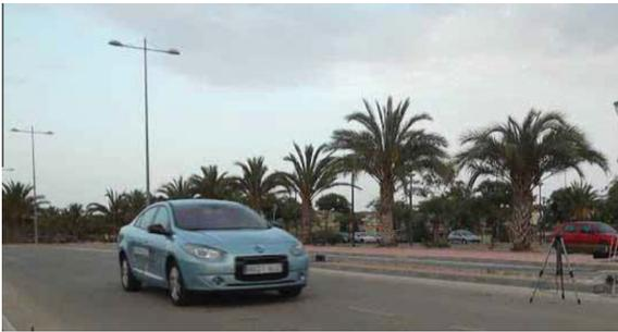
Fig. 1. Pass-by test of an electric vehicle.
