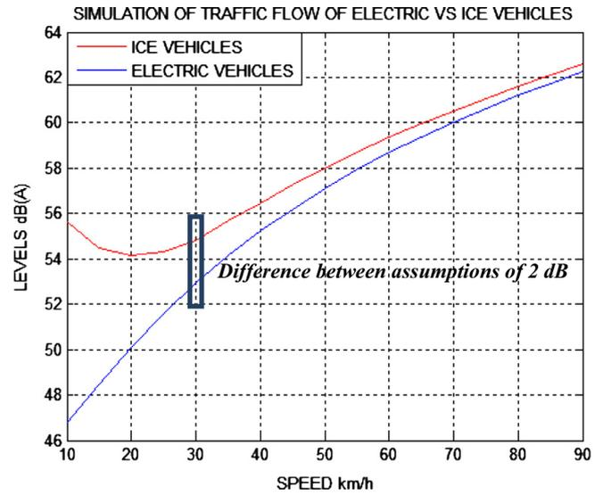
Fig. 5. Simulation of traffic flow of electric vs ICE vehicles.
